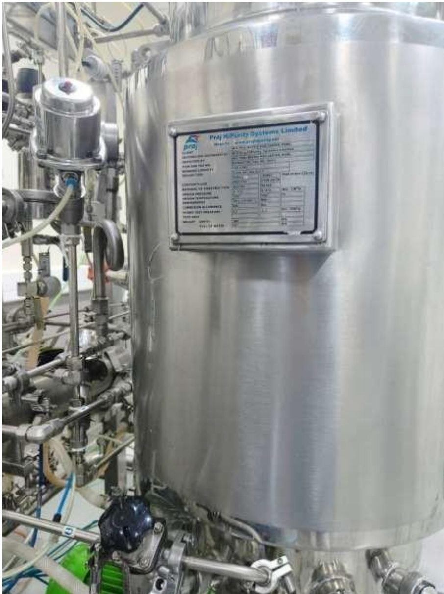
Fig 4.1. A typical 100 liter fermentor by Praj HiPurity Systems
