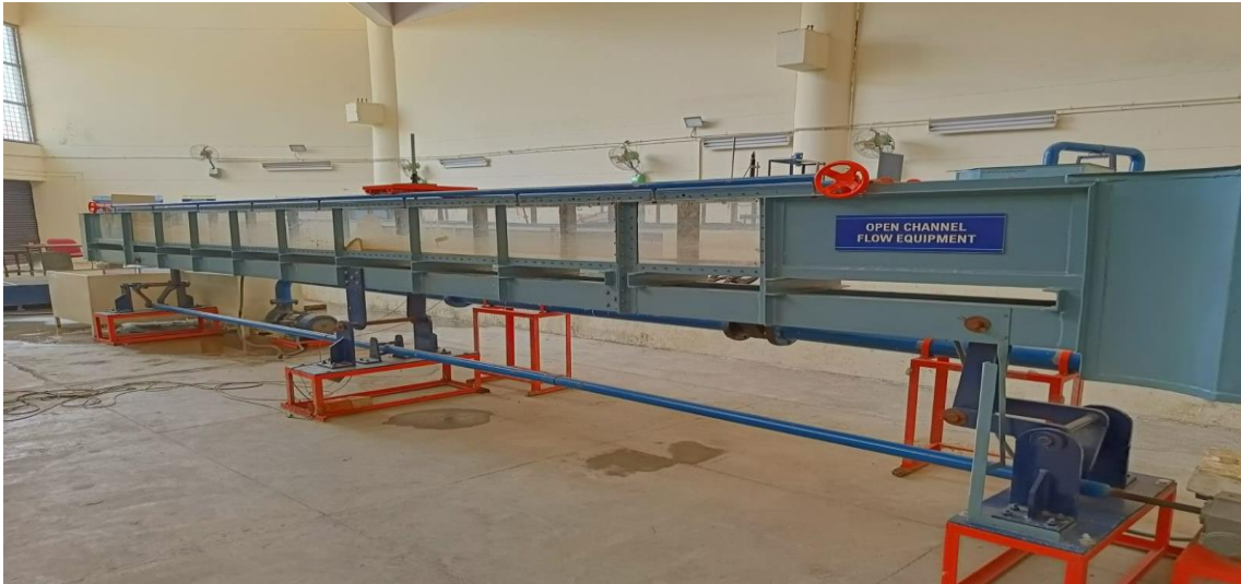
Figure 3.1. Rectangular tilting flume
