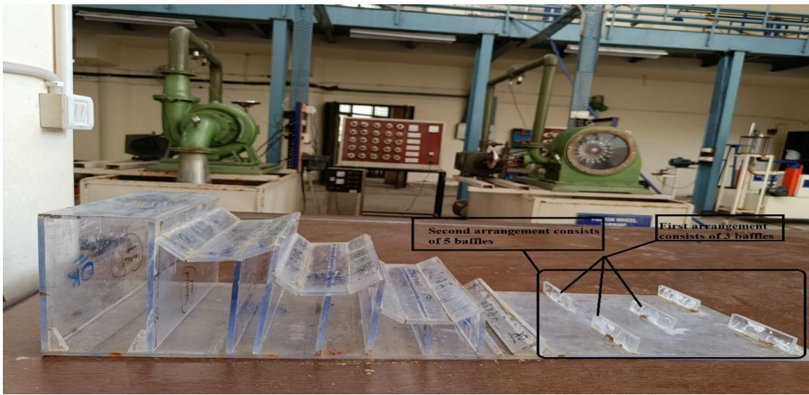
Figure 3.4. Arrangements of baffles in trapezoidal stepped spillway
