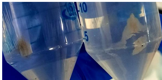
Figure 5: Ammonium sulphate precipitation pellets were observed at 40 % saturation after incubation period of 17 hours.
