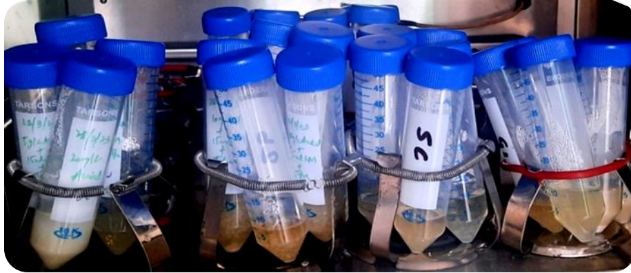
Fig 6: Experiment set up for cellulases production at different concentrations. Experiments were set up at 3 different concentrations of avicel i.e 0.5 %, 1 % and 2 %. Each concentration was set up with four biological replicates.
