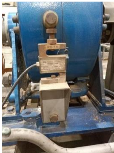
Plate 3.9: Load cell placed on the dynamometer
