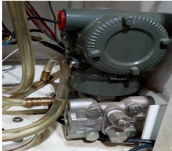
Plate 3.11: Fuel flow sensor
