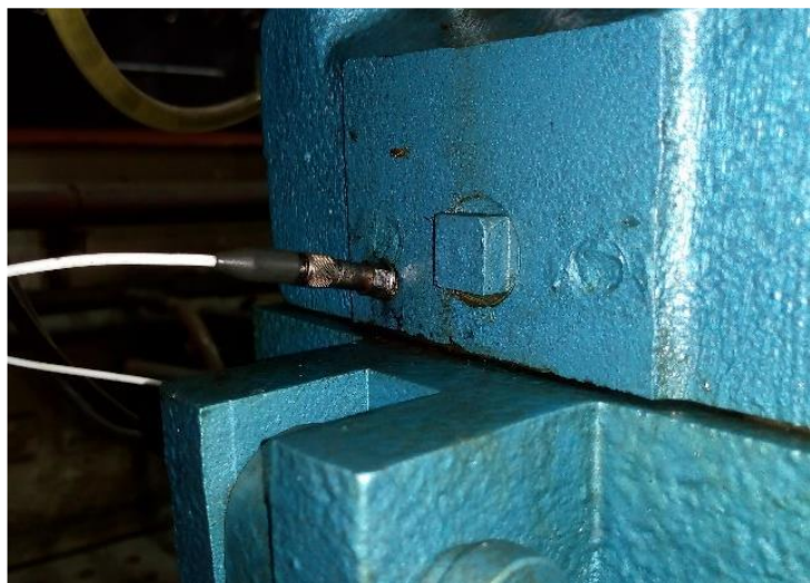
Plate 3.13: Pressure sensor installed on the engine head
