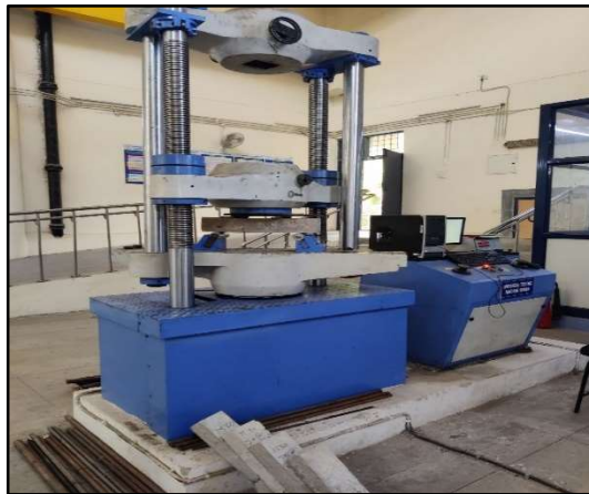
Figure 3. 7 Testing of Beams Using UTM
