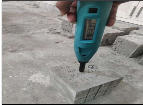
Figure 3. 5 Rebound Hammer Testing
