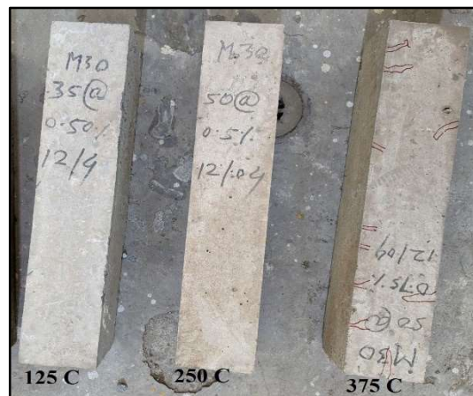
Figure 4. 5 Change in Color at Various Temperature
