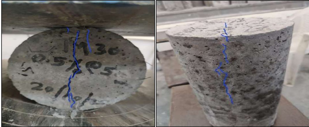
Figure 4. 4 Crack Pattern in Cylinder
