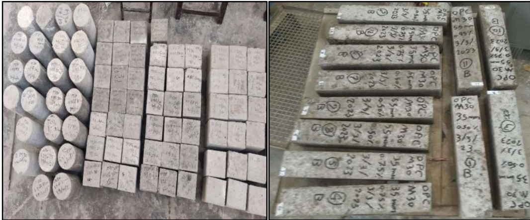
Figure 3. 4 Cubes, Cylinder, and Beams for Testing
