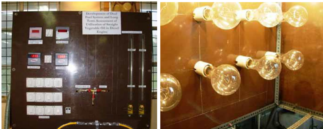
Plate 3.7: Control Panel & Load Bank
