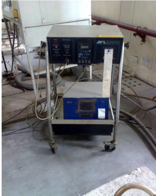
Plate 3.8: Smoke Meter and Di Gas Analyzer
