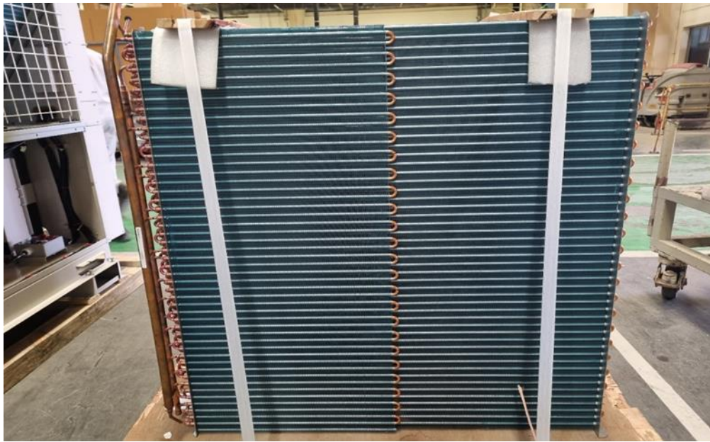
Figure 1.21.1 Pre-coated aluminum fin coils [19]
