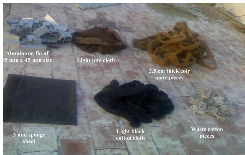
Figure 2.3 Demonstration of different wick materials.
