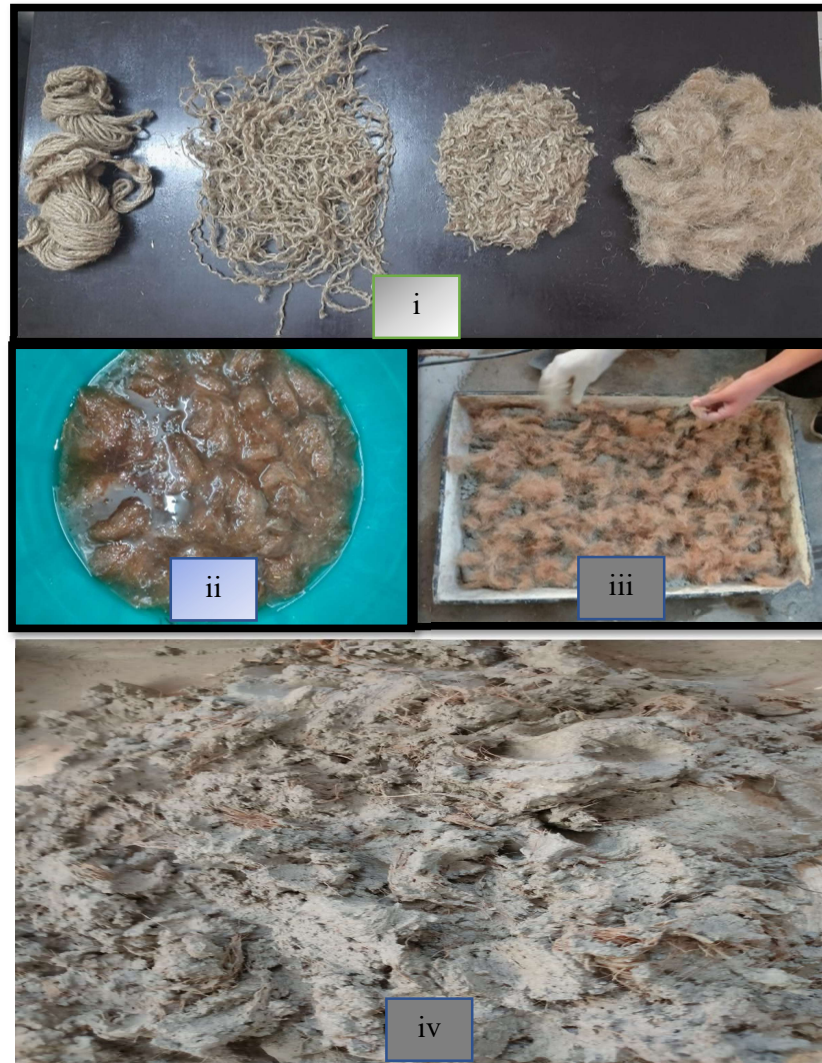
Figure 3.3. (i)Preparation of jute fibre, (ii)Water absorption test, (iii) Before mixing, (iv)After mixing
