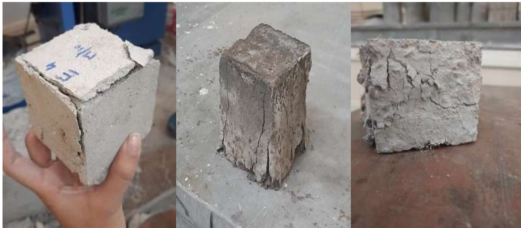
Figure 3.5. Failure of egg, jaggery, and jute mortar cubes, respectively
