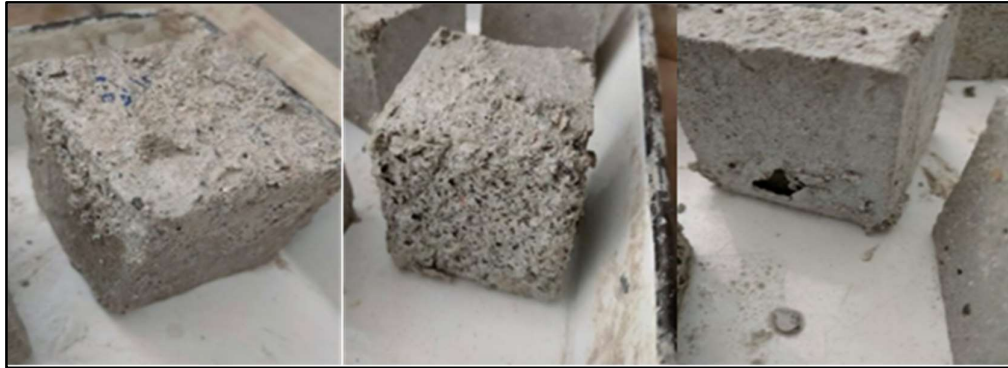
Figure 3.7. Cubes showing different type of failure after acid attack
