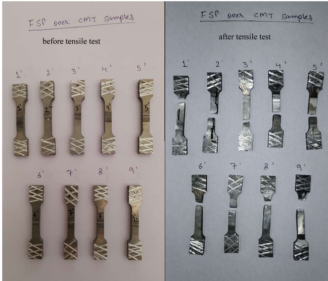
Figure 3.10. FSP over CMT samples before and after tensile test
