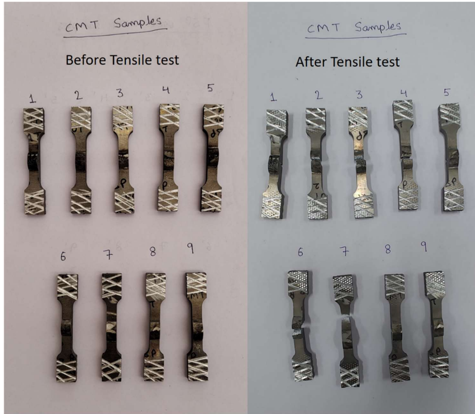
Figure 3.9. CMT samples before and after tensile test
