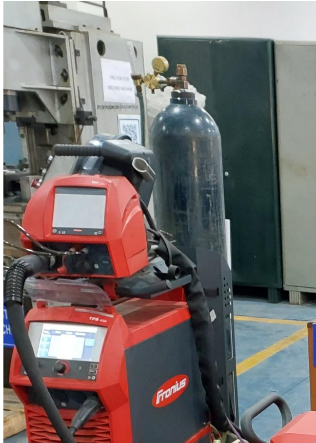
Fig. 3.2.2 CMT Power Source, Wire Pool, and Argon Gas cylinder
