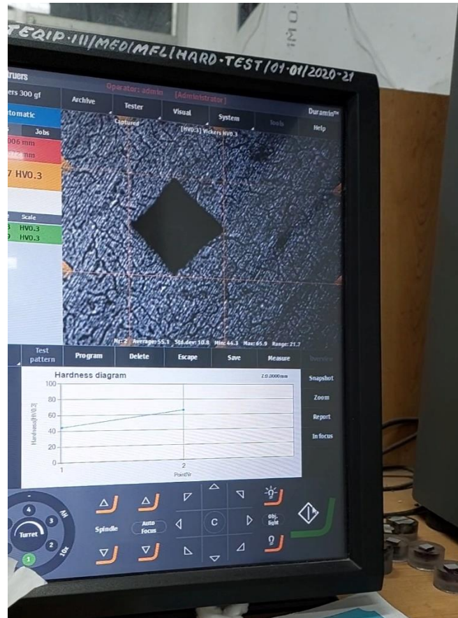
Fig. 3.3.3.3 Monitor showing indent
