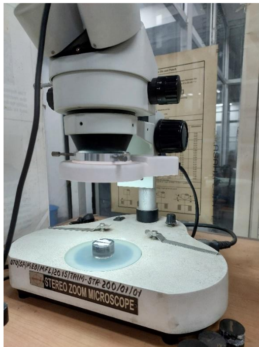
Fig. 3.3.1.1 Stereo Zoom Microscope, with mounted monolayer sample
