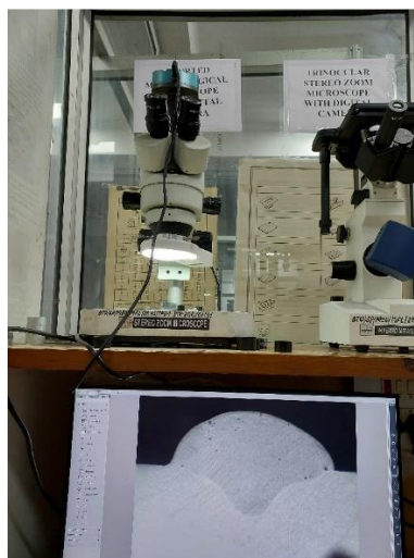
Fig. 3.3.1.2 Stereo Zoom Microscope with macro image shown on monitor
