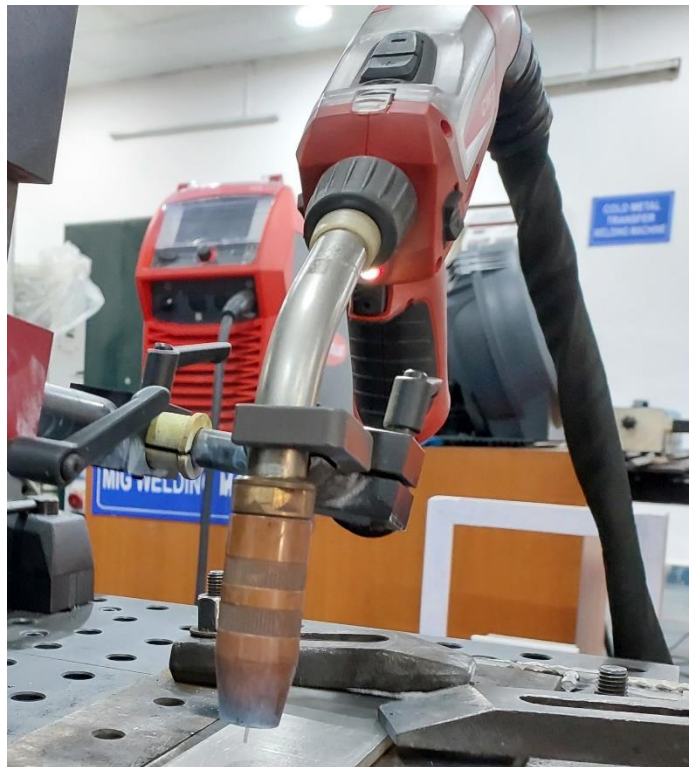
Fig. 3.2.3 CMT Torch, with Nozzle
