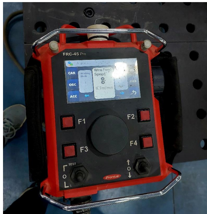
Fig. 3.2.5 Remote for controlling robotic motions and process parameters
