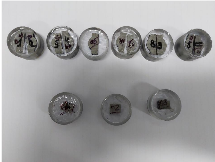
Fig. 3.6.1 Samples mounted for polishing
