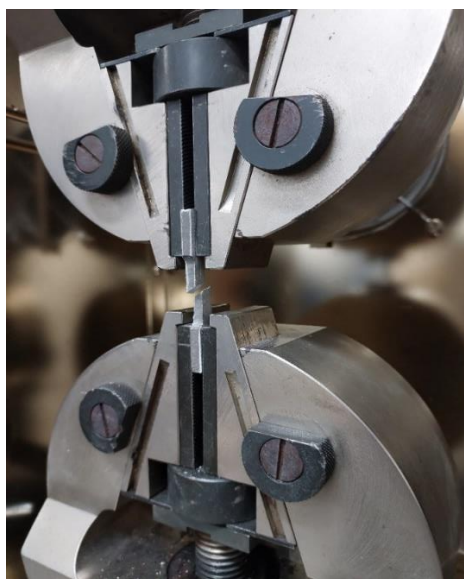
Fig. 3.3.2.2 Dog shaped sample after fracture on UTM
