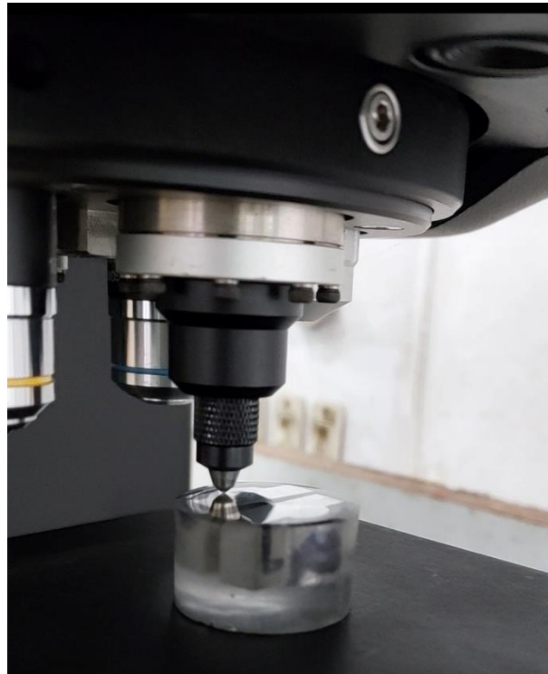
Fig. 3.3.3.2 Making indent on mounted monolayer cross section by Duramin 40 struers hardness tester
