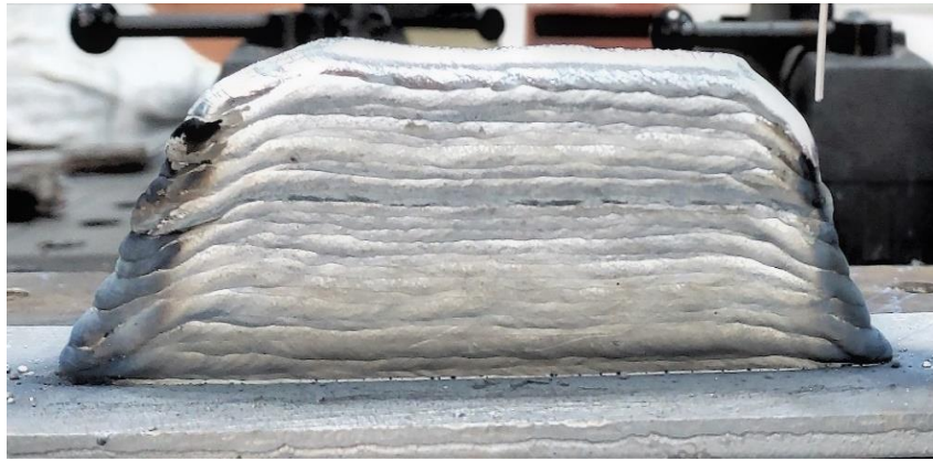
Fig. 4.3.1 CMT-WAAM made AA4047 wall
