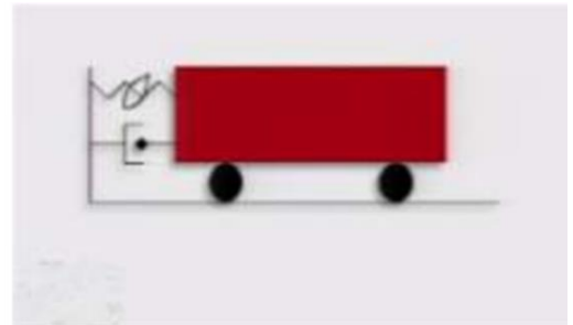
Fig. 10.2 SDOF oscillator with inelastic material behaviour
