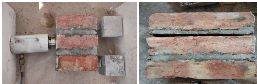
Figure 3.6. Brick Triplet before testing and after testing
