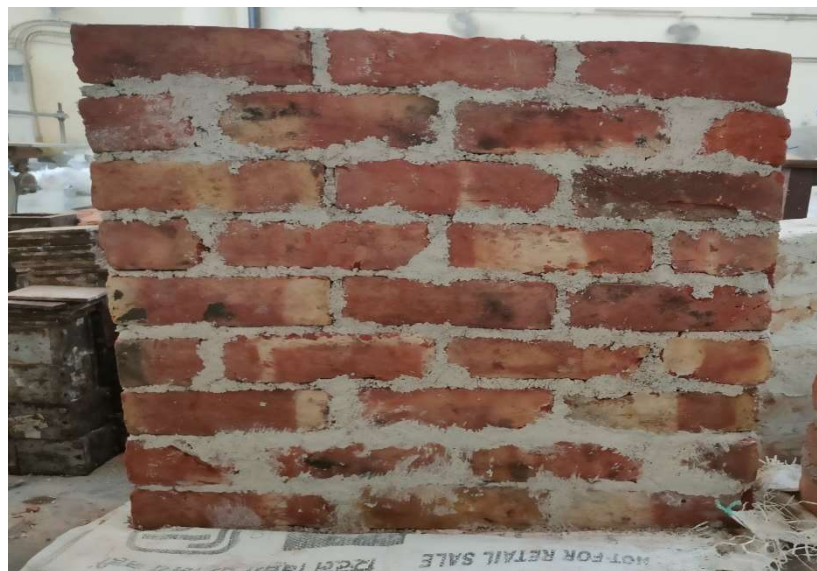
Figure 3.4. Masonry Wall for Diagonal Testing
