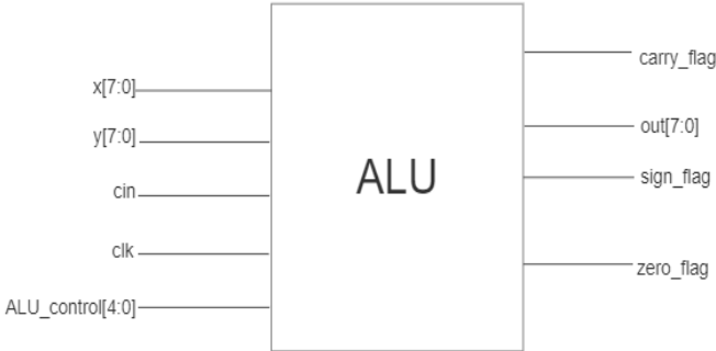
Fig 2.8 Block diagram of conventional ALU
