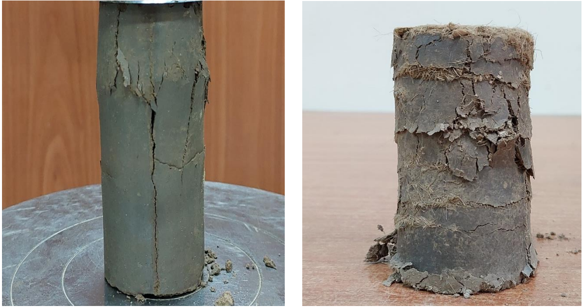
Fig. 5.16 Comparison between Unreinforced (left) and jute reinforced sample (2.5% f ) (right)
