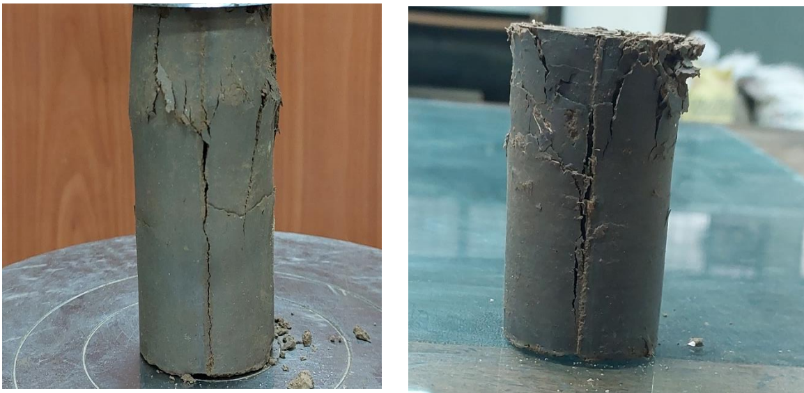
Fig. 5.6 Comparison between Unreinforced (left) and coir reinforced sample (2% f ) (right)
