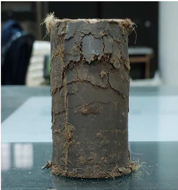
Fig. 5.20 Clockwise from top: 2% jute fiber reinforced soil; 2.5% jute fiber reinforced soil; 3% jute fiber reinforced soil.
