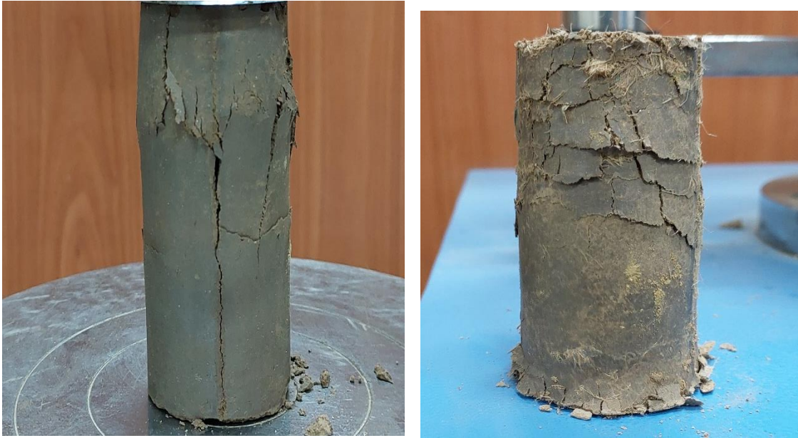
Fig. 5.18 Comparison between Unreinforced (left) and jute reinforced sample (3% f ) (right)
