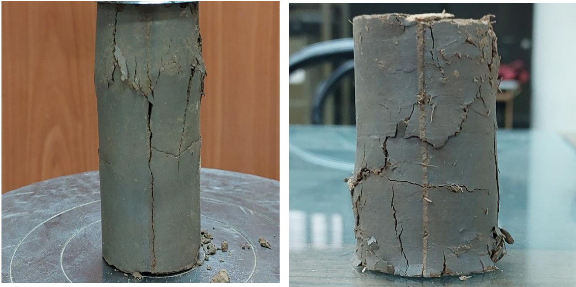
Fig. 5.8 Comparison between Unreinforced (left) and coir reinforced sample (2.5% f ) (right)
