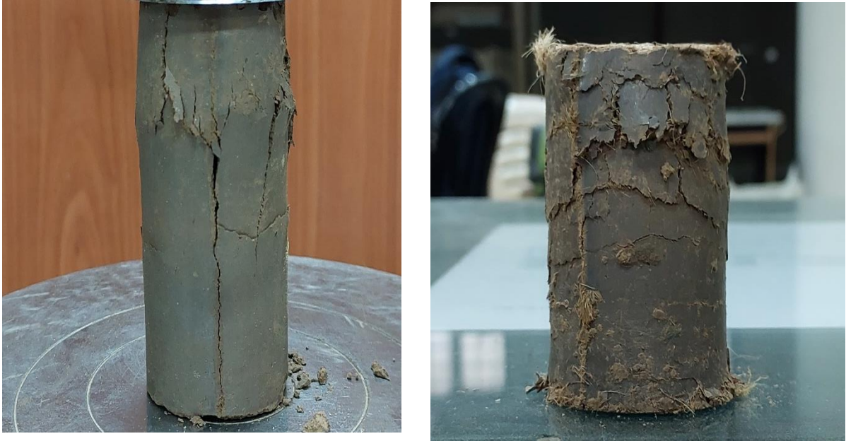
Fig. 5.14 Comparison between Unreinforced (left) and jute reinforced sample (2% f ) (right)
