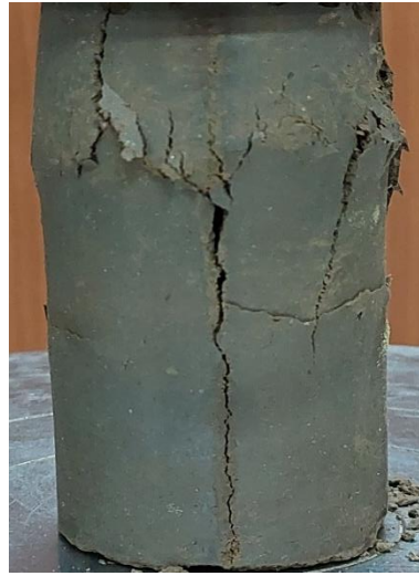
Fig. 4.2 Unreinforced Soil Sample before (left) and after testing (right)
