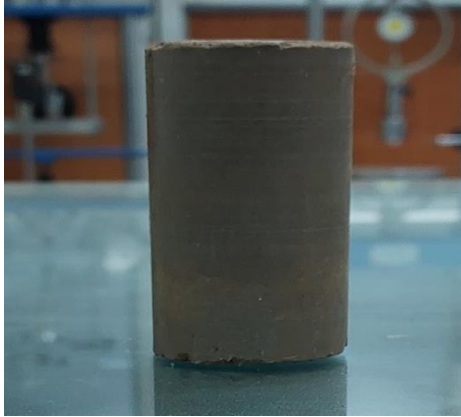
Fig. 4.2 Unreinforced Soil Sample before (left) and after testing (right)
