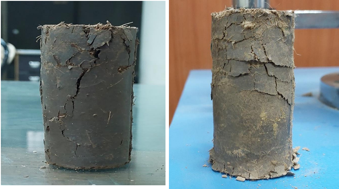
Fig. 5.22 Comparison between Coir Reinforced (3% f ) (left) and Jute reinforced sample (3% f ) (right)
