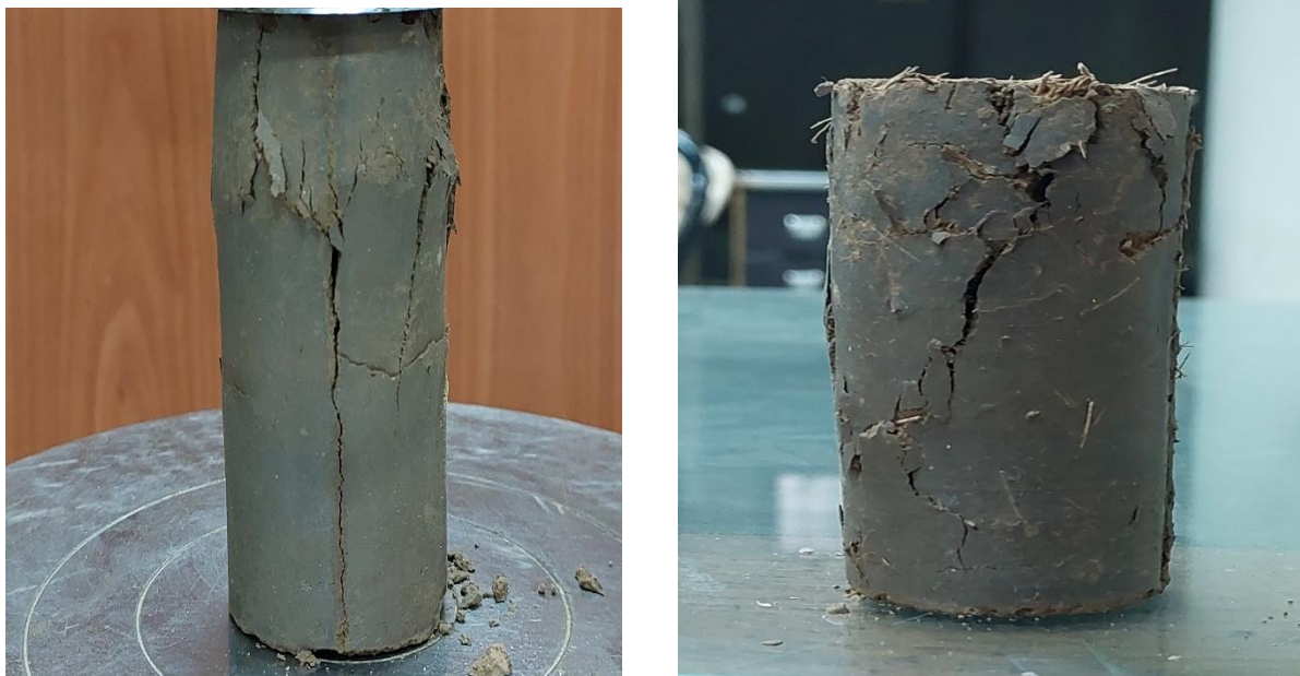
Fig. 5.10 Comparison between Unreinforced (left) and coir reinforced sample (3% f ) (right)
