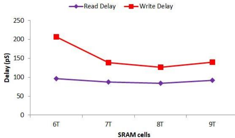
Fig. 5.3: Comparison of Read and Write delay of SRAM cells with varying transistor counts
