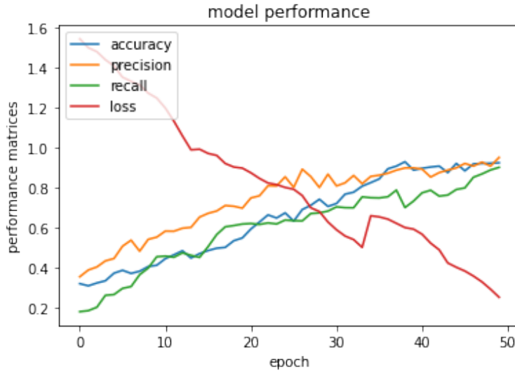
Figure 6.8: Performance Evaluation of the Proposed model using RMSprop with Nesterov Momentum Optimizer on Plant Pathology 2021-FCVG8 Dataset[14]
