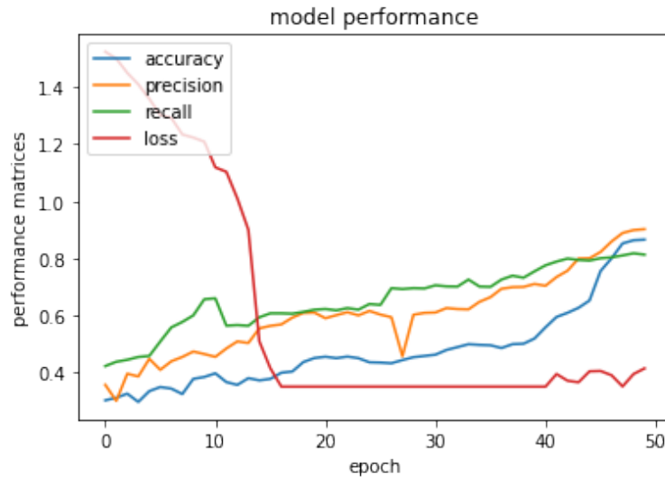
Figure 6.6: Performance Evaluation of the Proposed model using Nesterov Accelerated Gradient Optimizer on Plant Pathology 2021-FCVG8 Dataset[14]
