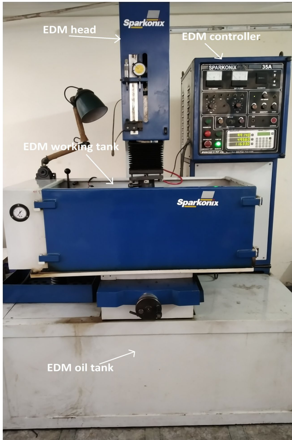
Figure 3.1. Conventional EDM machine (Sparkonix 35A).
