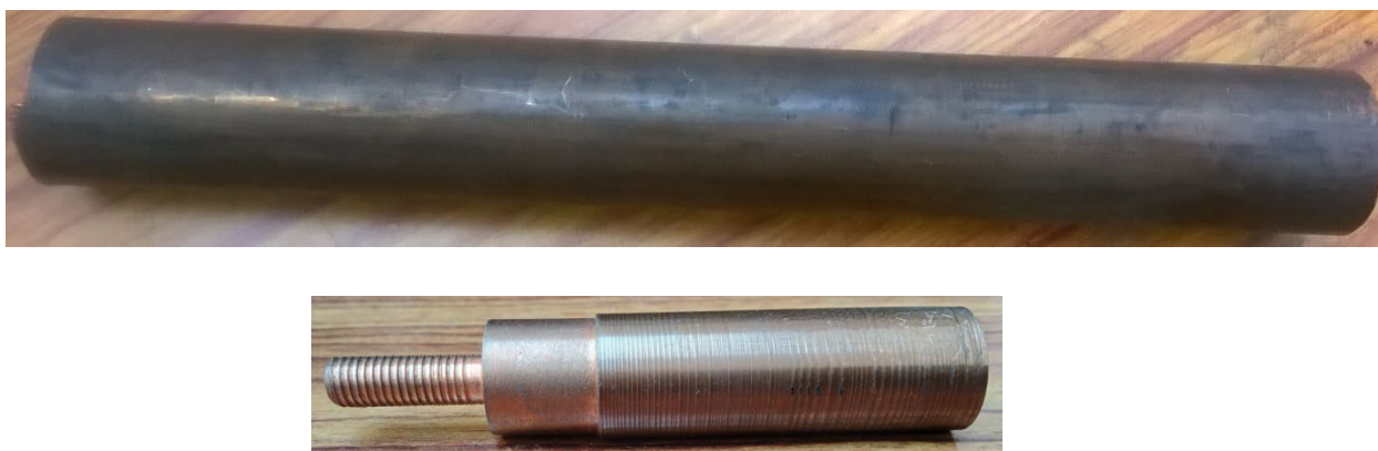
Figure 3.10. Before and after images of copper tool.
