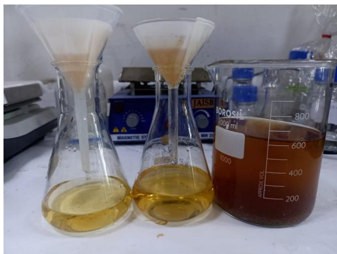
Fig.3.4 Failed filtration of potato sample
