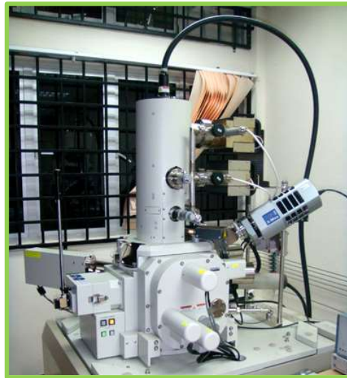
Fig. 3.2. Field Emission Scanning Electron Microscope (FESEM) Setup
