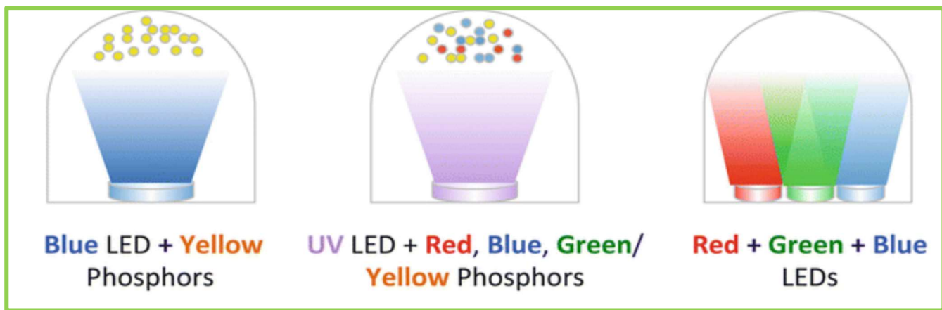
Fig. 1.2: White-light generation representation using phosphors
