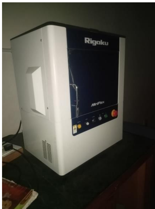
Figure 3.1. XRD machine, Rigaku Diffractometer (Mini flex 600, Japan)
