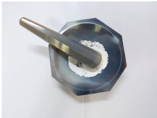
Figure 1.2. Solid state method used to form powdered Gd_2Ti_2O_7
