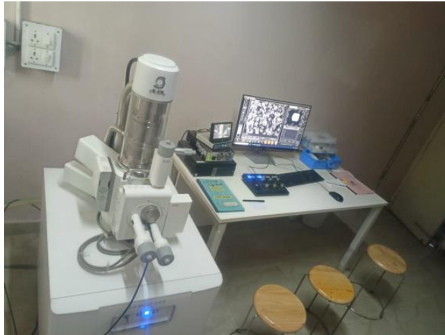
Figure 3.3. Scanning electron microscopy (SEM-JSM-IT 200, JEOL)
