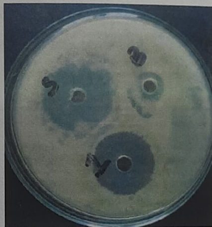
Figure 7: A representative picture of an agar plate demonstrating areas where CuNPs-applied S.Aureus growth was inhibited.
