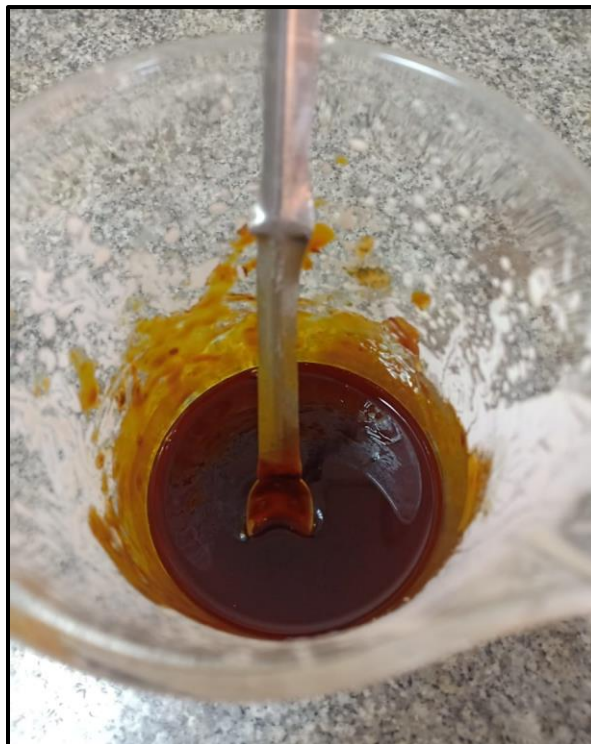
Fig10. Viscous adhesive formation on addition of NaOH
