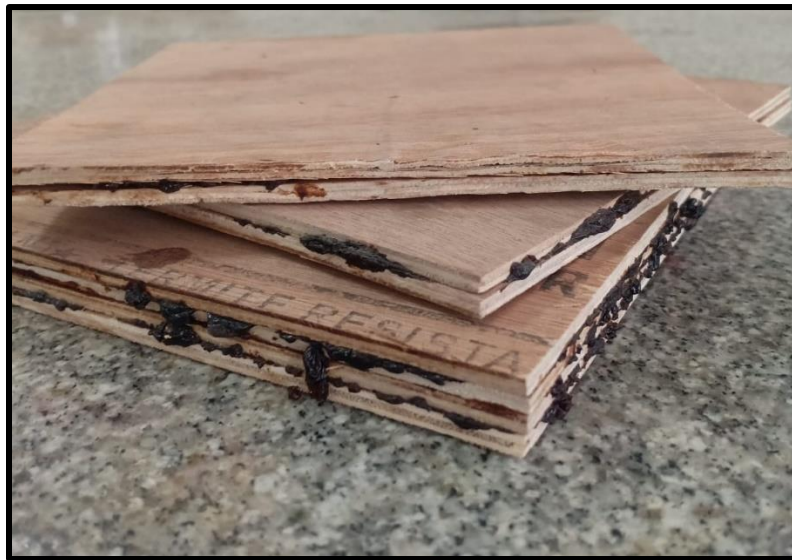
Fig11. Plywood panels adjoined together using our adhesive
