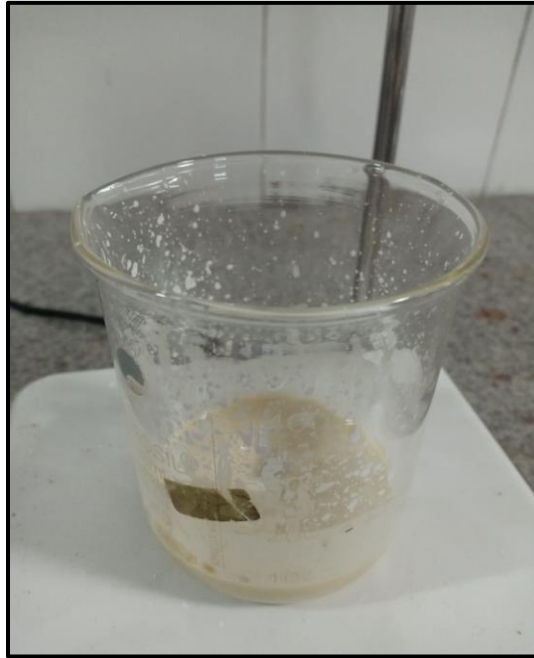
Fig9. Adhesive formulation on mixing cornstarch and tannin
