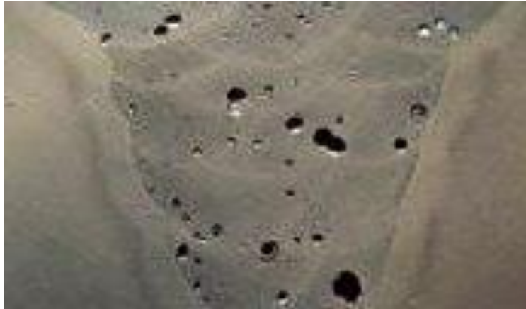
Figure 1.5: Porosity defect in aluminum weld joint [10]
