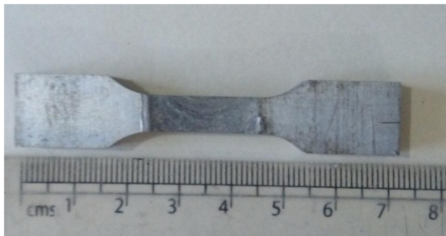
Figure 4.15: Tensile sample as per ASTM-E8 standard
