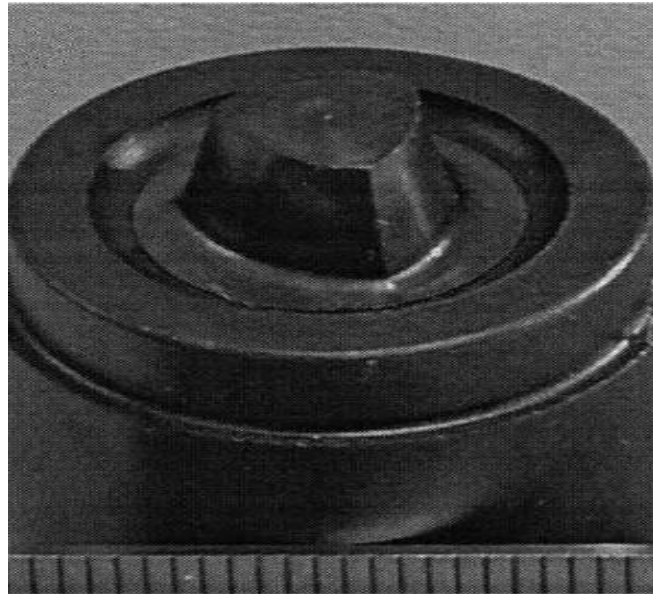
Figure 1.10: Design of thread less pin [39]
