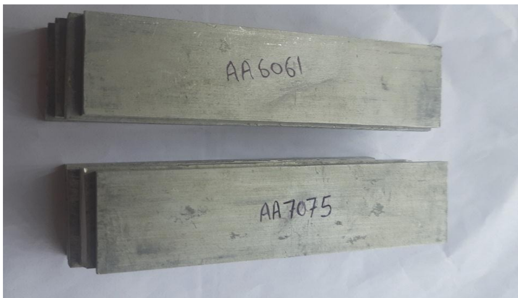
Figure 4.2: Base plates of AA 6061 and AA 7075
