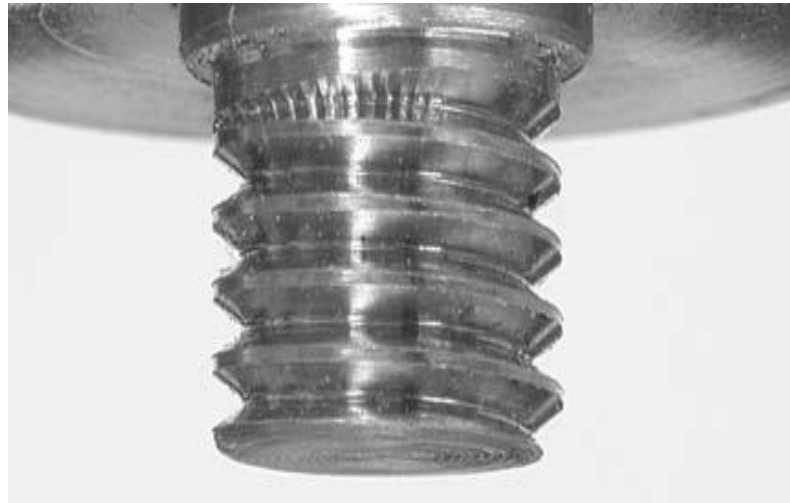
Figure 1.8: Design of flat bottom cylindrical pin [37]
