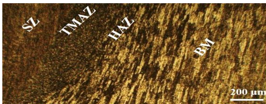
Figure 5.17: Optical graph of various zones of FSPed composite joint of AA6061 and AA7075
