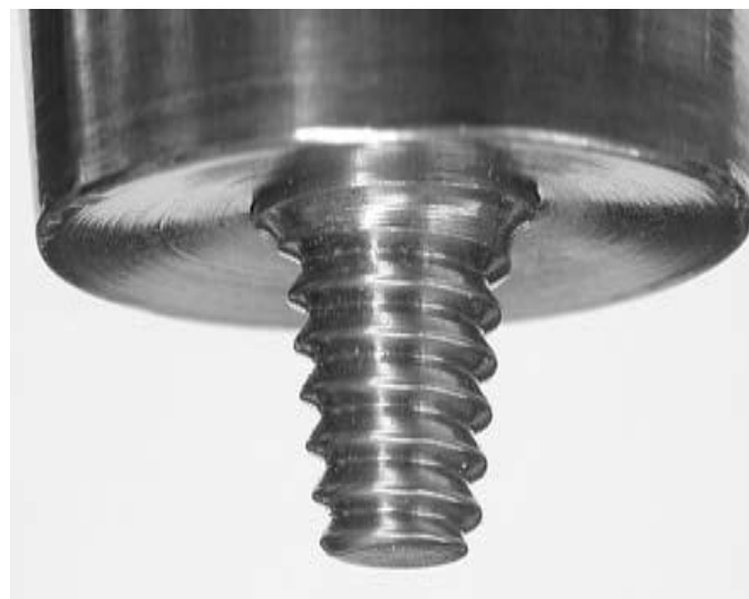
Figure 1.9: Design of truncated cone pin [38]
