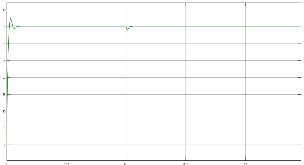
Fig 7.30: Voltage at output of POSLLC under SMC with change in load resistance.
