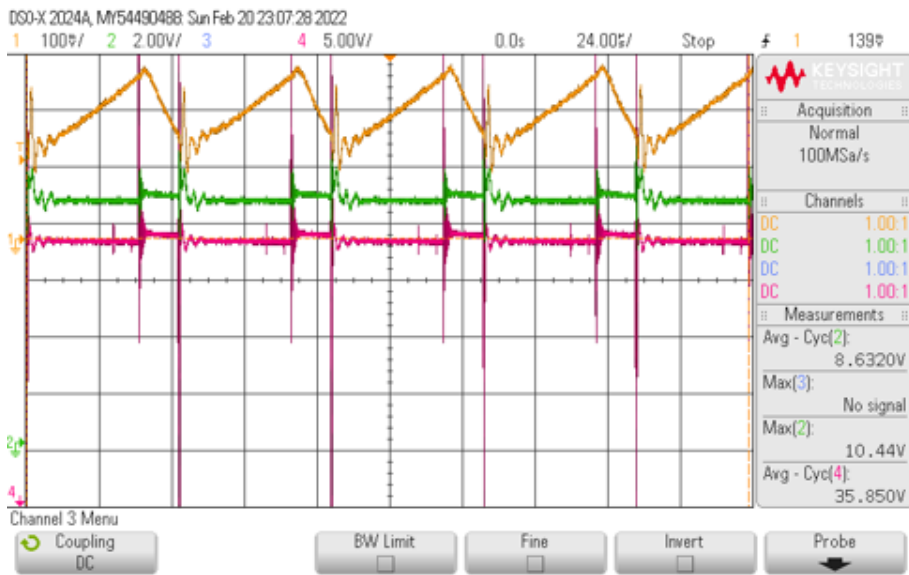
Figure 7.3: Total output voltage, V_{o1} and inductor current at 50 kHz
