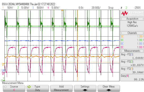
(c) output waveforms when Sampling frequency is equal to switching frequency at f_s = 50\text{kHz}
