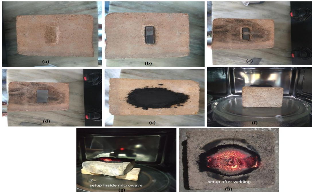
Fig.4.14: Step wise procedure of microwave welding
