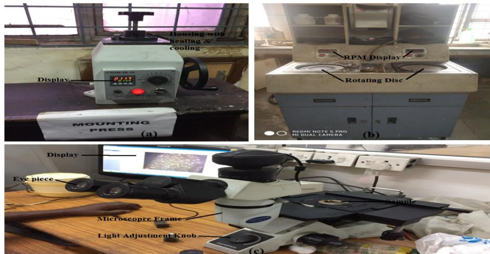
Fig.4.17: a) mounting press, b) polishing machine, c) optical microscope
