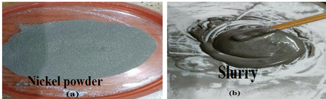
Fig.4.7: a) Nickel powder, b) Nickel powder mixed with epoxy resin
