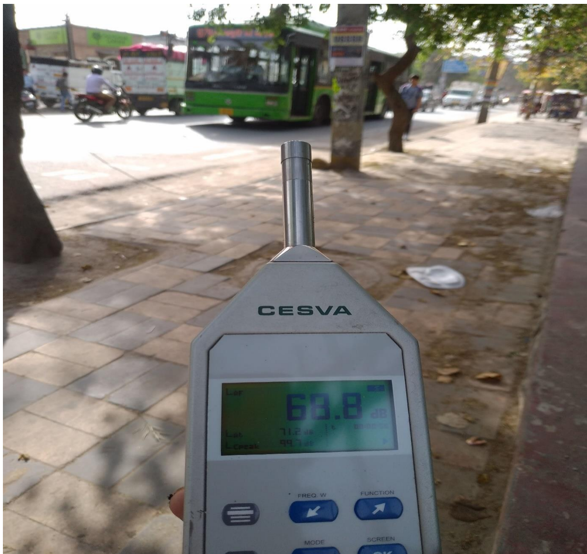
Figure 3.17 Roadside Noise Monitoring at D.T.U
