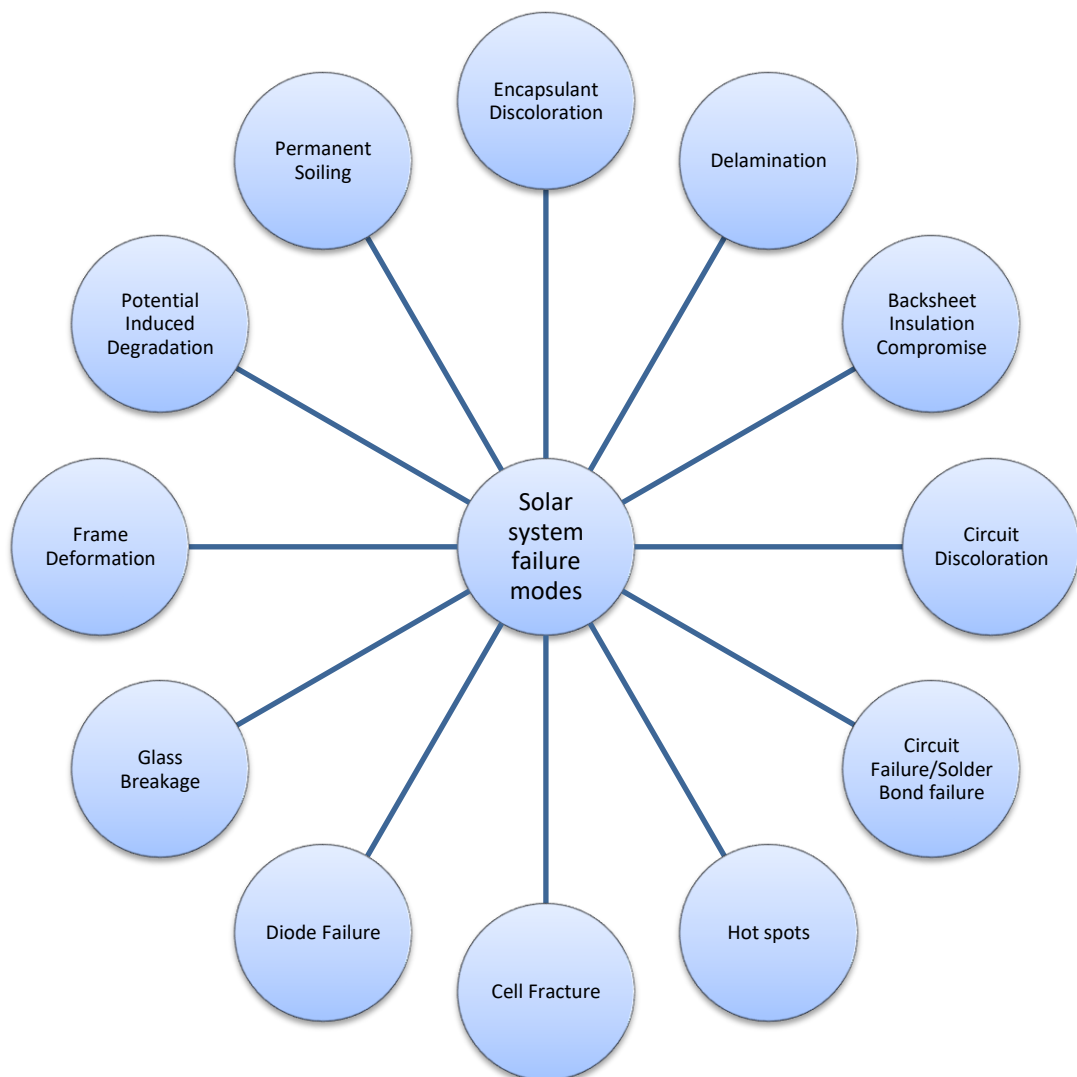
Figure.5.1 Failure modes of solar system
