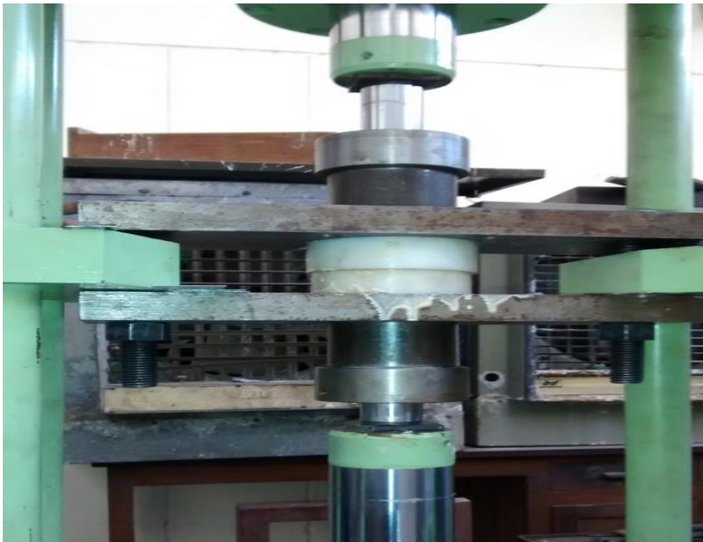
Fig 4.7. Photograph of developed AFM set up
