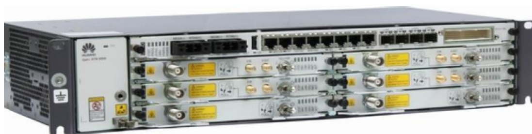
Figure 3 2 A view of microwave IDU used in for the new Microwave backhaul
