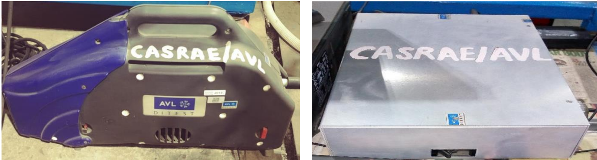
Plate 3.21. AVL DISMOKE smoke meter and AVL DITEST gas analyser
