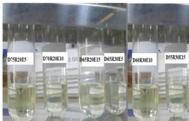
Plate 3.4. Ternary fuel samples blends of Diesel, Renewable diesel and ethanol
