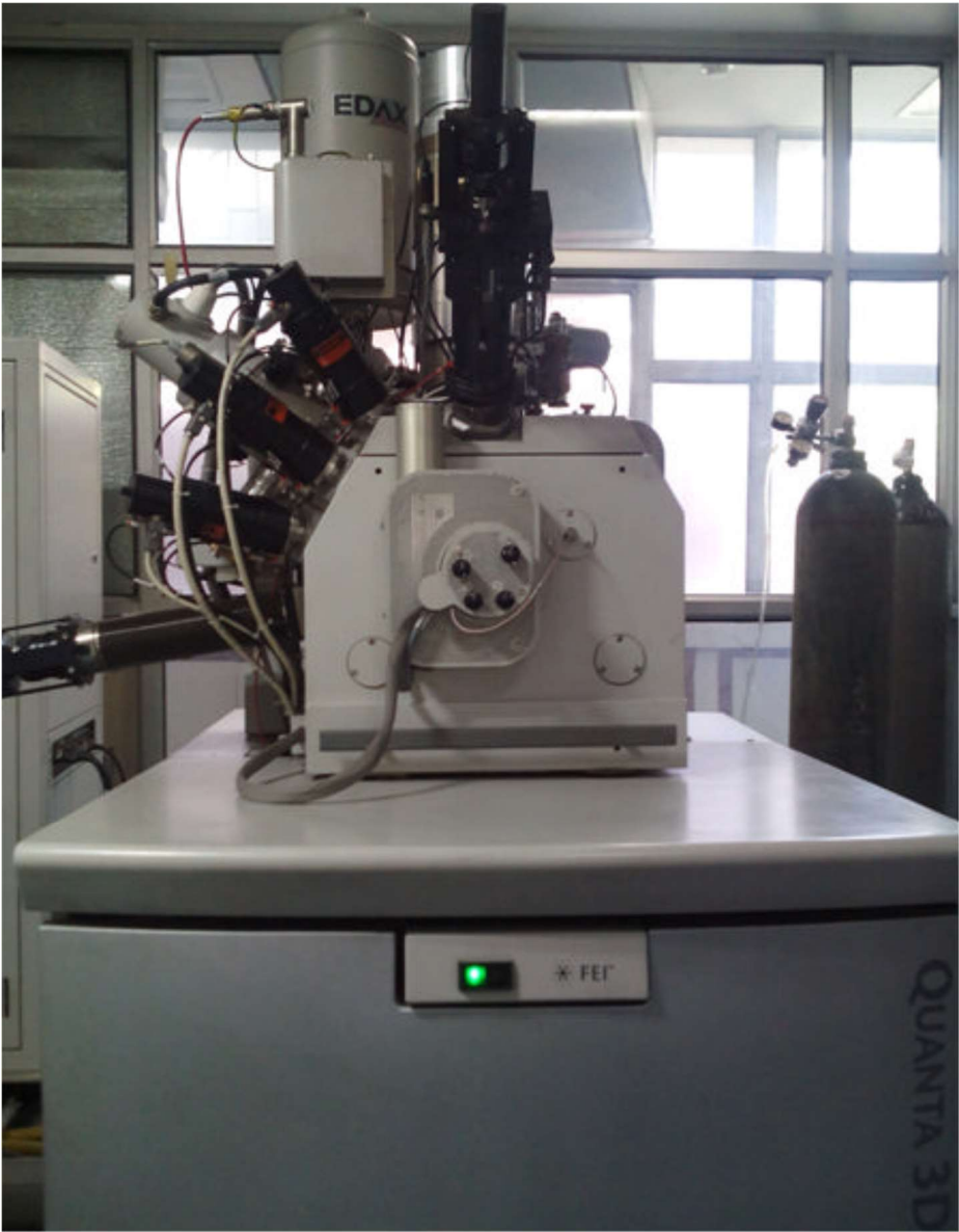
Fig. 3.7 Field Emission Gun Scanning Electron Microscope (FEG-SEM) (Model: FEI QUANTA 3D FEG)
