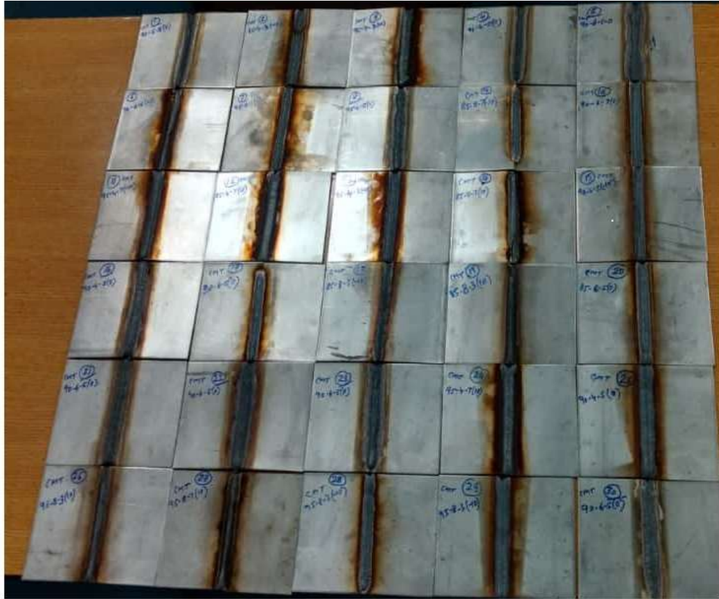
Fig. 3.12 CMT welded samples as per design matrix
