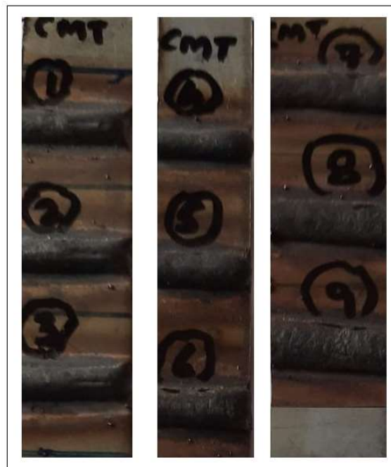
Fig. 3.11 CMT weld bead samples as per design matrix
