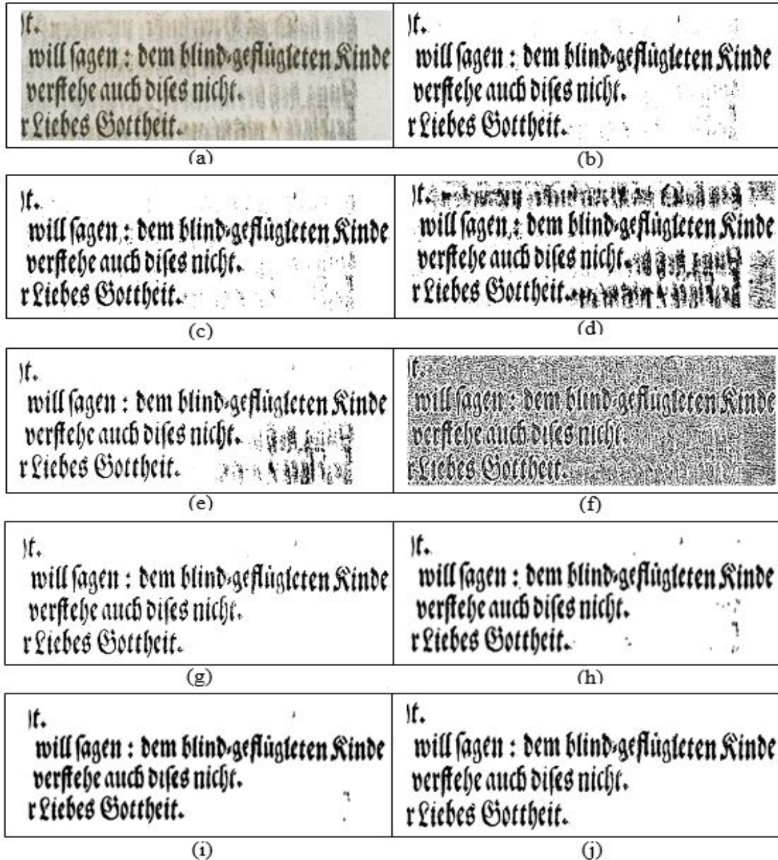
Figure 3.5: Comparison of binarization results; (a) Degraded image [124], (b) Otsu [6], (c) Sauvola and Pietikainen [11], (d) Niblack [8], (e) Singh et al [13], (f) Bernsen [14], (g) Lu et al [12], (h) Mitianoudis and Papamarkos [18], (i) Bhowmik et al [136], and (j) Proposed MLP-based method.
