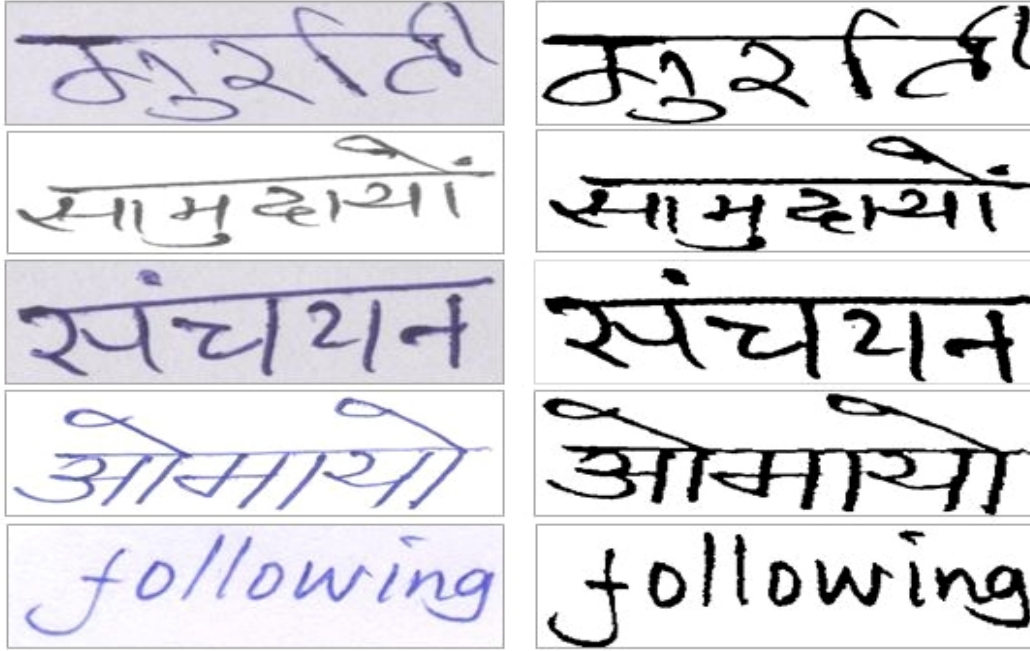
Figure 4.9: Normalization of word images by local centered-slant correction method. Left column shows skewed word images and right column are their respective normalized and binarized word images
