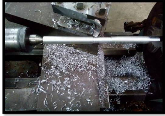
Figure 3.16 Tensile test specimen preparation on a conventional lathe machine
