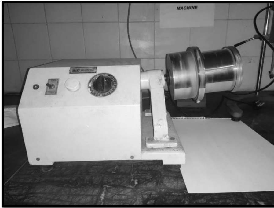
Figure 3.10 Ball mill machine set-up
