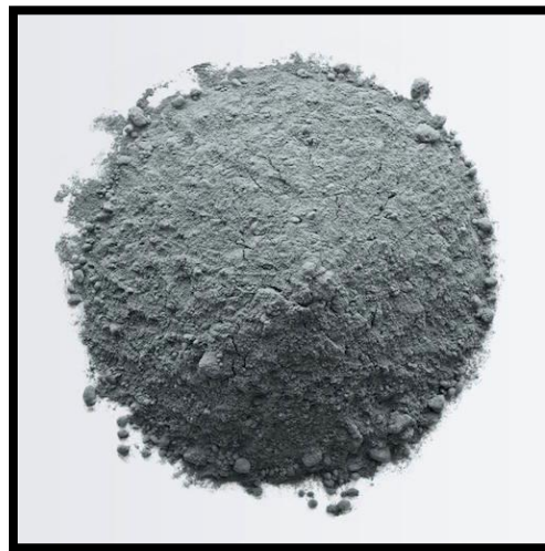
Figure 1.2 A class-F raw fly ash sample [3]
