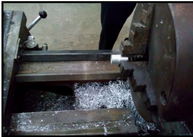
Figure 3.17 Compression test specimen preparation on a conventional lathe machine
