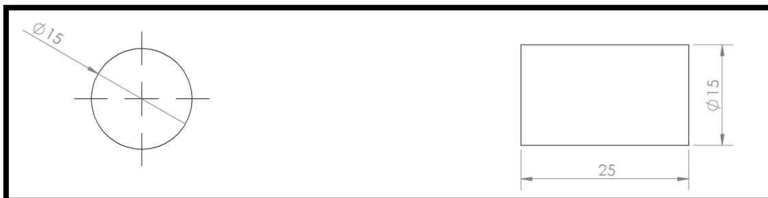
Figure 3.13 Dimension of compression test specimen
