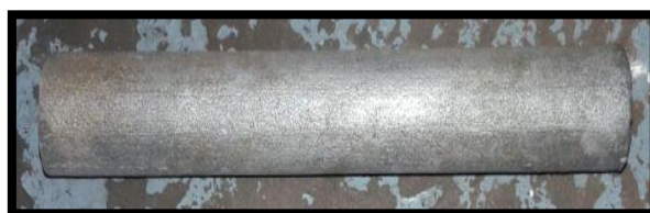
Figure 4.4 Un-machined Stir-casted Cylindrical Rods
