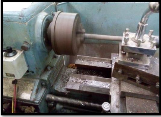
Figure 3.16 Tensile test specimen preparation on a conventional lathe machine
