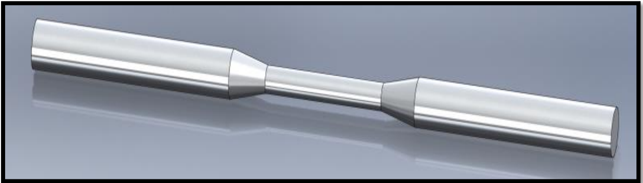
Figure 3.14 CAD for tensile test specimen
