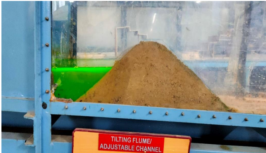
Figure 4.1: M1- Homogeneous earth dam
