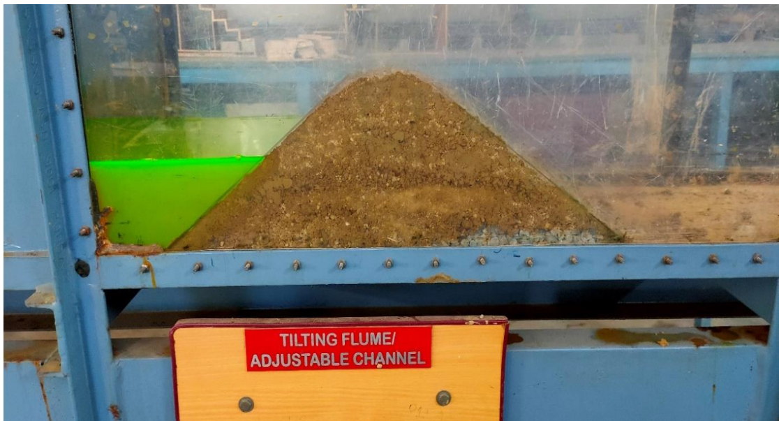
Figure 4.3: M13- Earth dam with downstream filter
