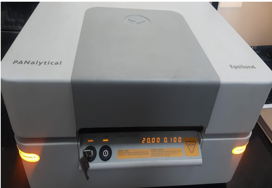
Figure 24: Malvern Panalytical Energy Dispersive X-ray fluorescence (EDXRF) spectrophotometer model Epsilon 4, made in the United Kingdom
