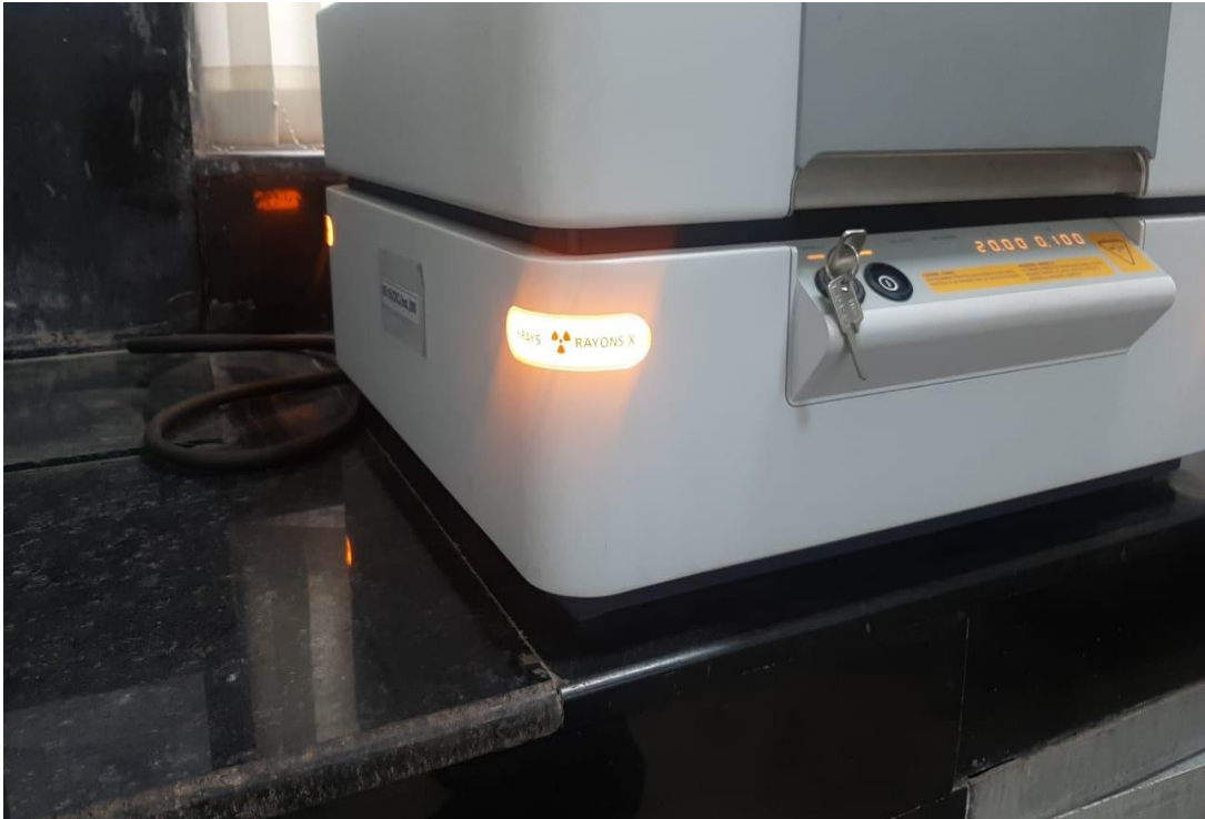
Figure 23: Malvern Panalytical Energy Dispersive X-ray fluorescence (EDXRF) spectrophotometer model Epsilon 4, made in the United Kingdom
