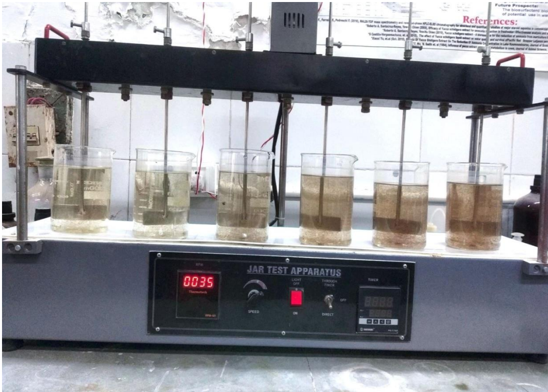
Figure 27: Experimental setup after the flocculation process of wastewater using composted cow dung
