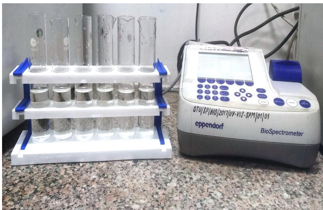
Figure 19: Nitrate nitrogen- Spectrophotometric set-up
