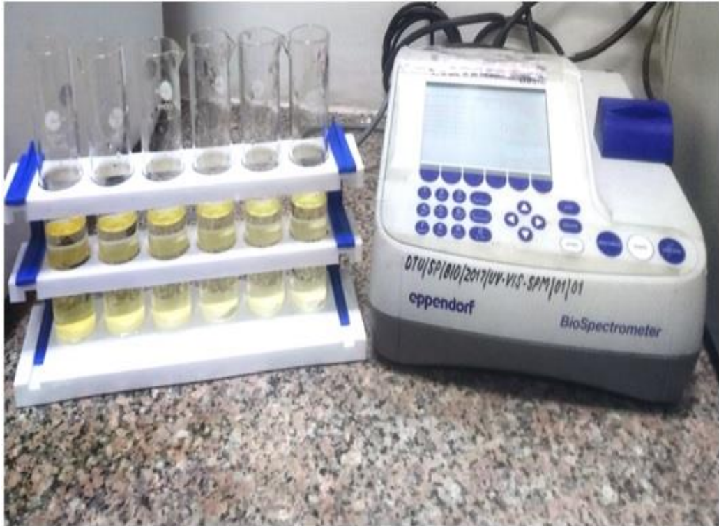
Figure 16: Ammonia nitrogen- Spectrophotometric set-up
