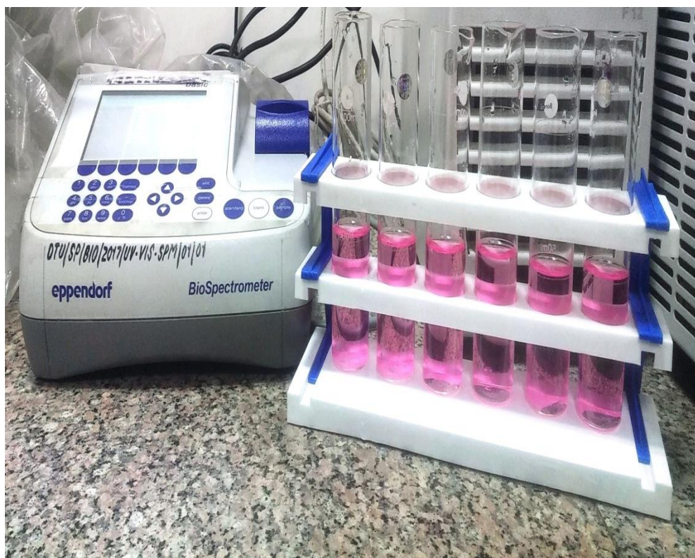
Figure 18: Nitrite-nitrogen- Spectrophotometric set-up
