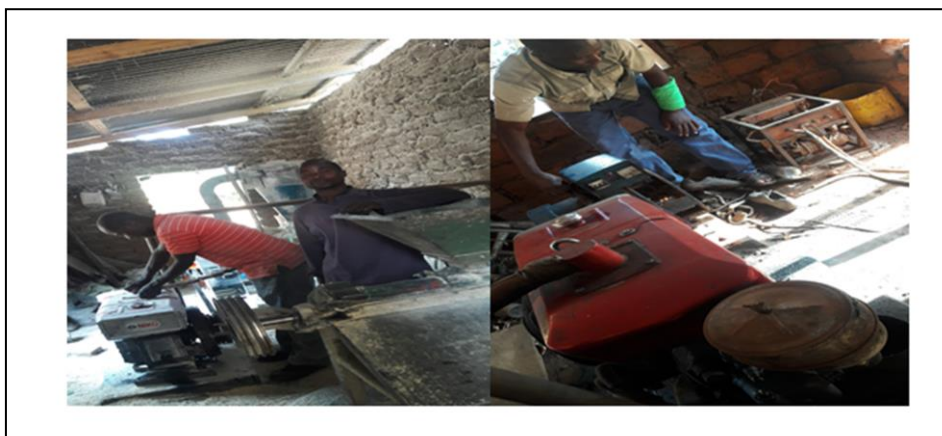
Figure 1.9. Maize flour/huller milling machine driven by diesel (Left side) and local fabricated diesel power plant for welding activities, lighting, and charging mobile phones (Right side) at Ikukwa residents (Source: By author)
