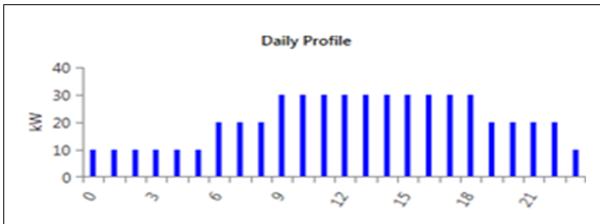
Figure 7.8. Electrical load over a 24-hour period simulated by HOMER pro software
