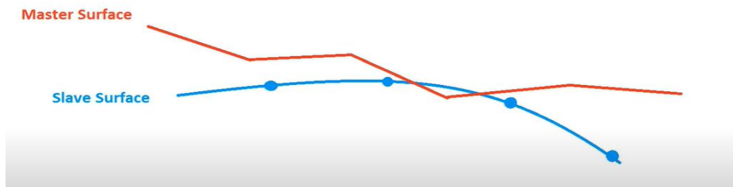
Figure 3.11: Master and slave surfaces
