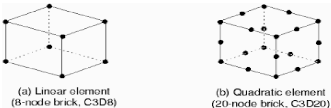
Figure 3.3: Linear and quadratic elements
