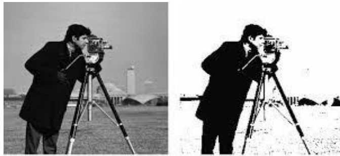
Figure 8. Segmented Image using Fuzzy C-Means (FCM) Clustering
