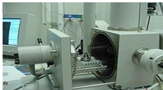
Figure 12: SEM with opened Chamber
