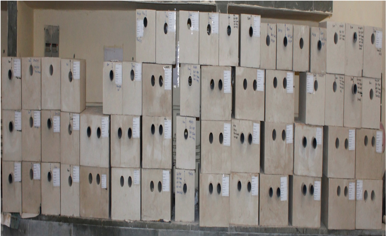
Fig. 4.11 Rock Tunnels Model prepared for experimental analysis.
