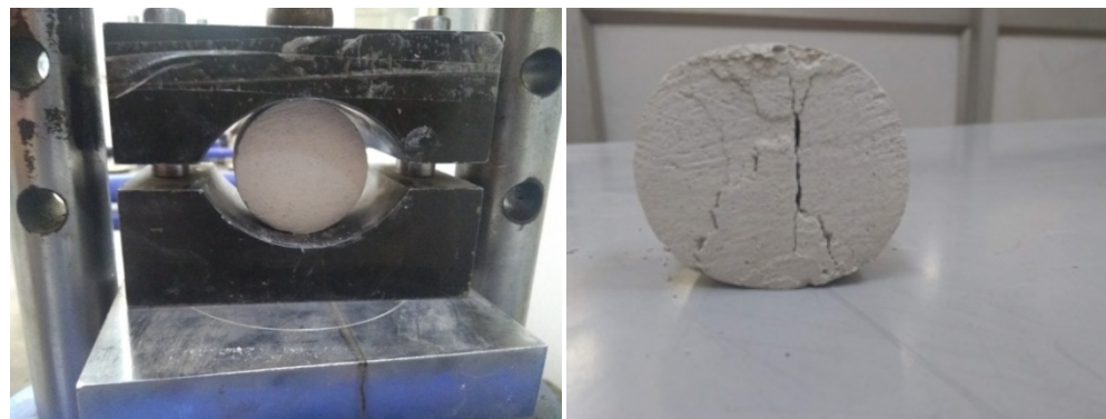
Fig. 4.5 Deformed UCS specimens after testing
