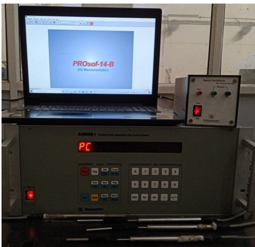
Fig. 3.6 Close Up View of Data Acquisition System
