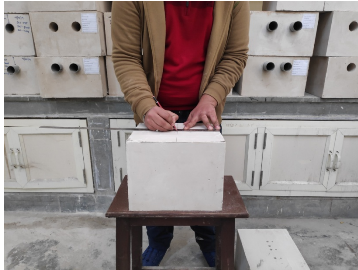
Fig. 4.12 Marking the dimensions on the bottom of the tunnel sample
