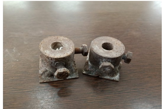
Fig. 3.12 Tri-nut system for fixing LVDT inside the tunnel sample
