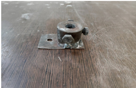
Fig. 3.12 Tri-nut system for fixing LVDT inside the tunnel sample
