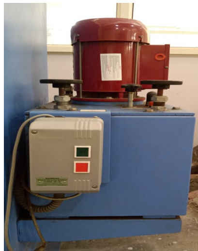
Fig.3.4 Pumping Unit attached to the loading unit.
