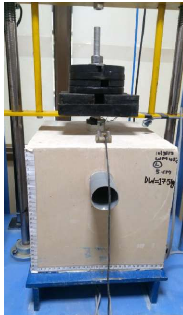
Fig.2.23 Rock Tunnel models having different coverdepths (Sharma et al. 2018)
