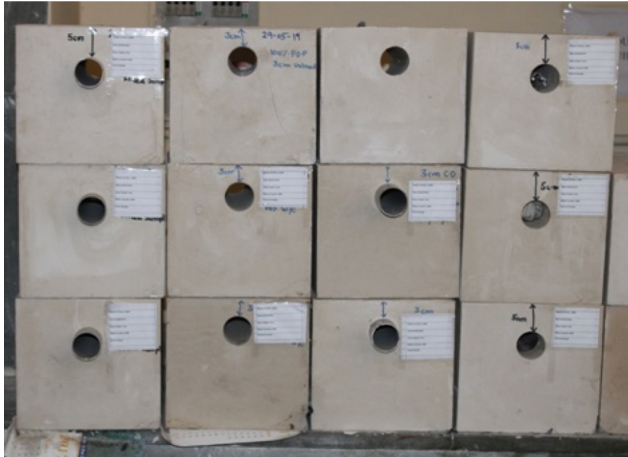
Fig. 4.9 Single lined and unlined tunnel samples with different cover depths
