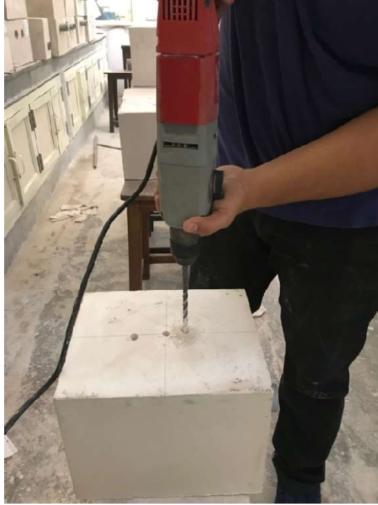
Fig. 4.13 Drilling holes inside the tunnel sample
