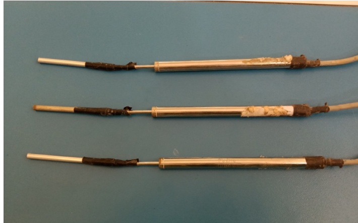
Fig. 3.11 Extension fixed to LVDT for fixing inside the tunnel sample
