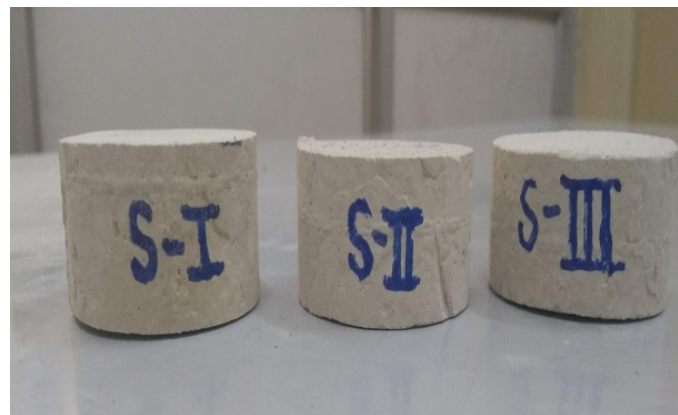
Fig. 4.3 Specimens of different Geomaterials prepared for Brazilian test to determine the indirect tensile strength.
