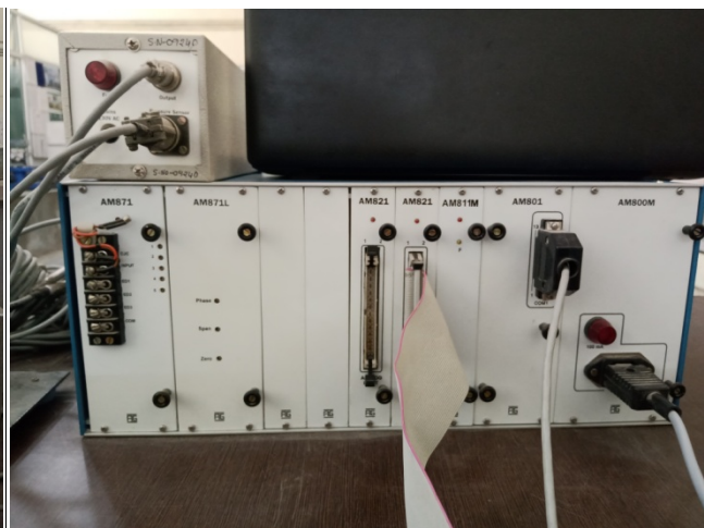
Fig. 3.7 Close Up of Rear View of LVDT Data Logger
