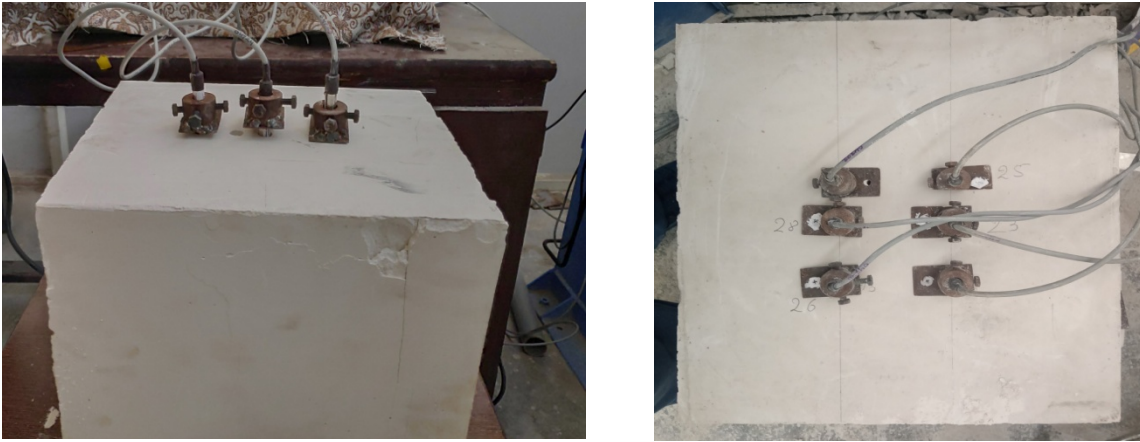
Fig. 3.13 Placement of LVDT inside the tunnel sample
