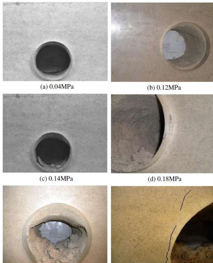
Fig. 2.20 Experimental results of gradual failure.
