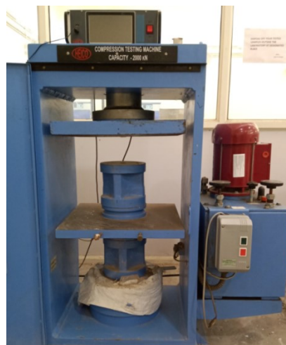
Fig. 3.2 Compression testing machine with an electronic display unit and pumping unit.
