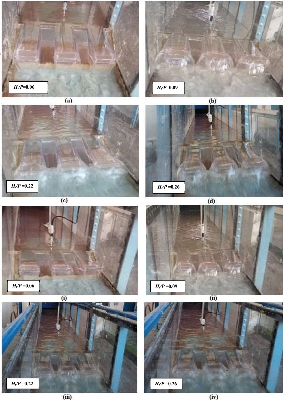
Figure: 4.4 Surface tension effects to jet trajectory formation from (a) to (d) on Largest models and from (i) to (iv) on Smallest models.
