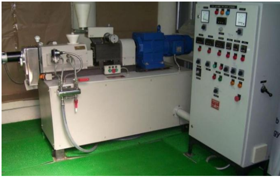
Fig.5. Twin-Screw Extruder has been used for the preparation of fish diets.
