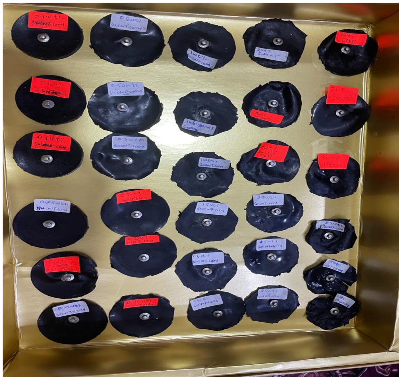
Figure 5.12: Electrodes of various concentrations of SWCNT-COOH/PDM
