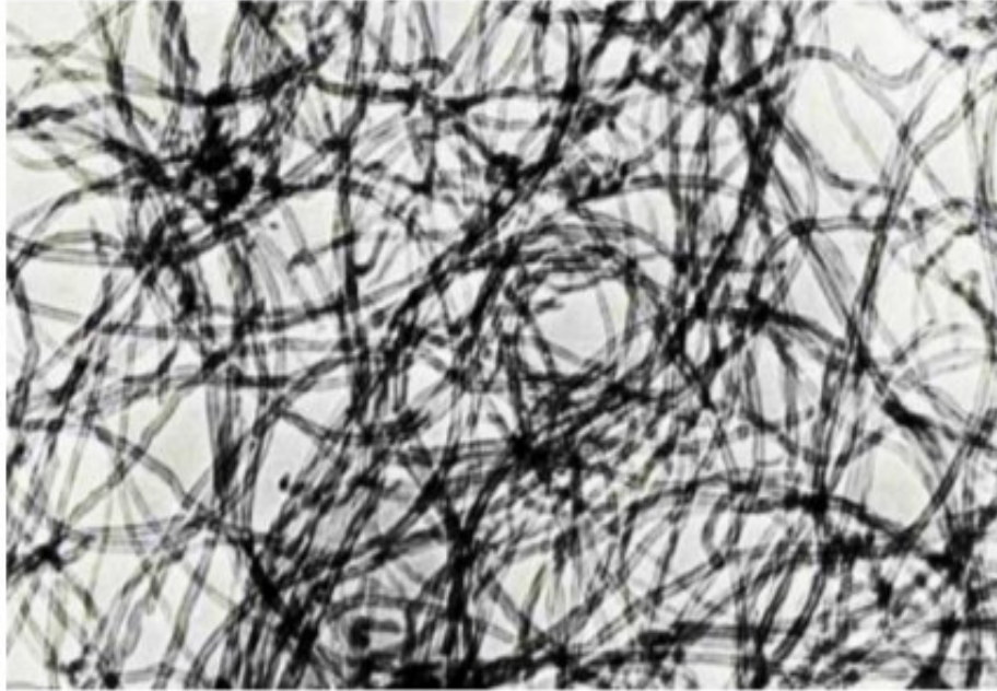
Figure 5.14: TEM of SWCNT-COOH
