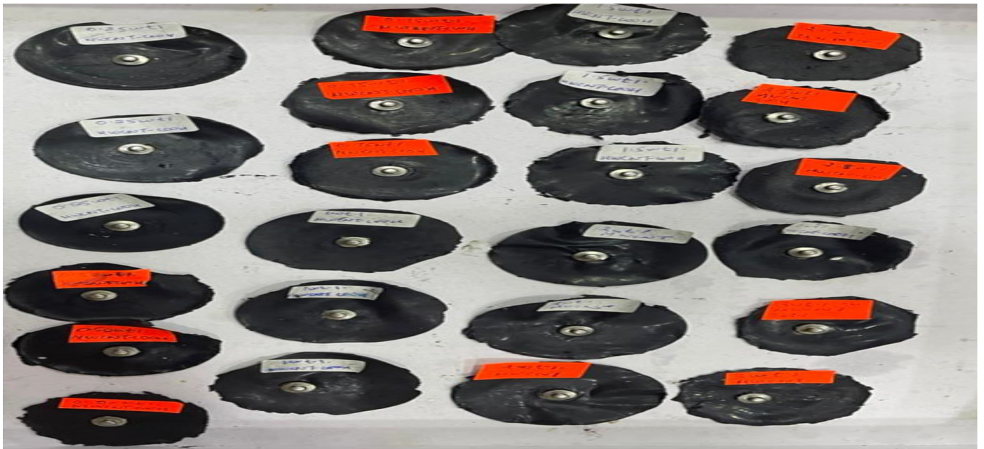
Figure 5.5: Electrodes of various concentrations of MWCNT-COOH/PDMS
