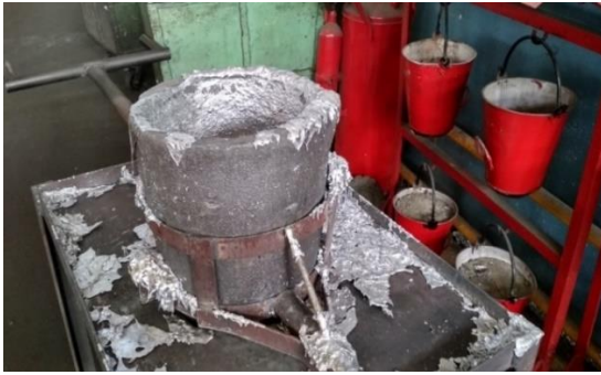
Fig. 1.10 Ladle carrying molten aluminum
