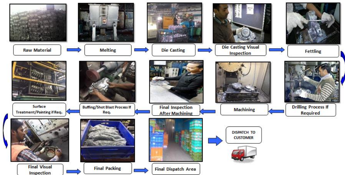
Fig. 1.9 General process sequence for crankcase covers manufacturing
