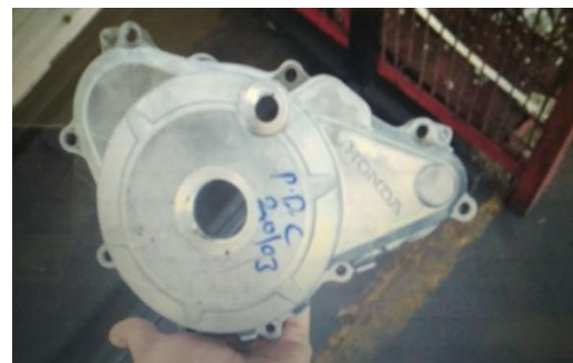
Fig. 5.2 Cover left crankcase K38
