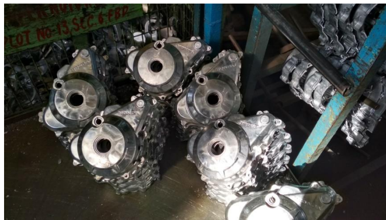
Fig. 1.12 Crankcase covers obtained through PDC machine
