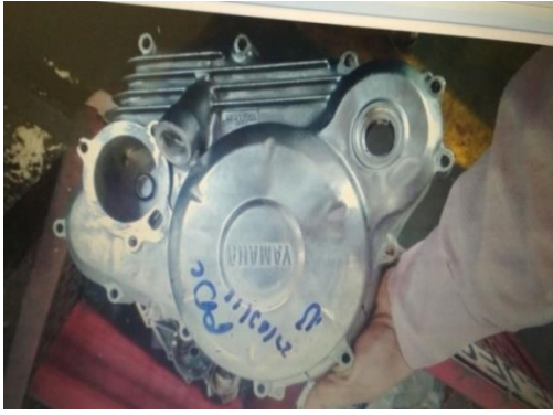
Fig. 5.3 Cover crankcase 206 G
