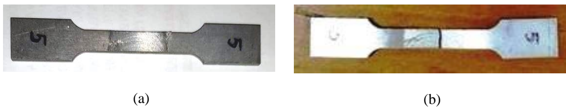
Figure 3.13 Specimen for tensile test before and after
