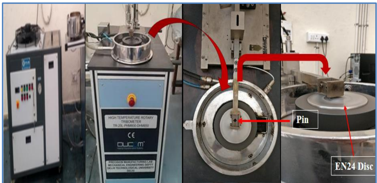
Figure 3.16 Experimental set up for wear test
