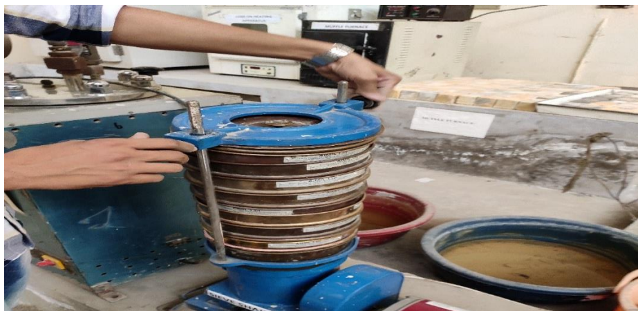
Fig – 11 Sieve shaking of fine aggregate
