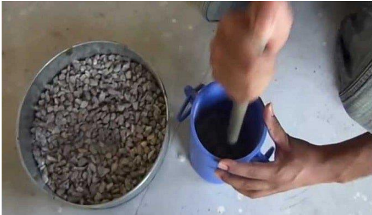
Fig –8 Aggregate crushing test
