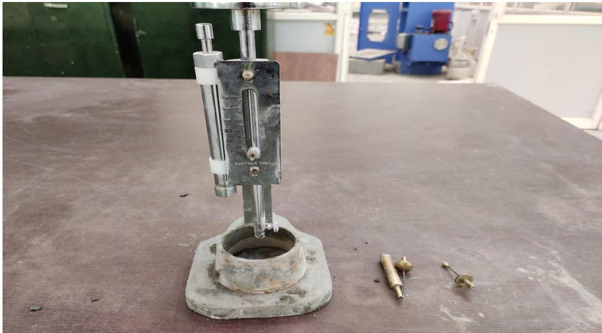
Fig – 6 Vicat apparatus showing different needles
