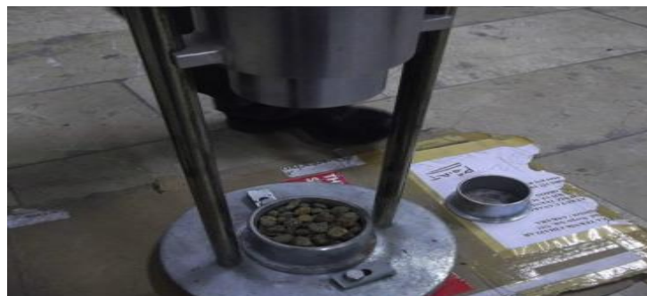
Fig – 9 Impact test of aggregate
