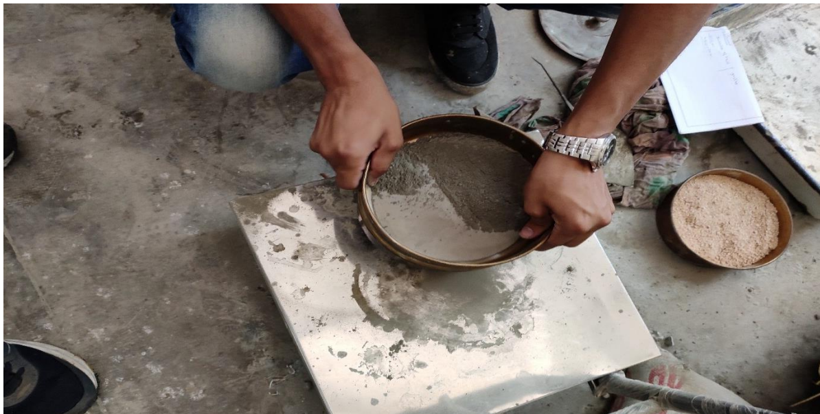
Fig – 5 Dry sieving of cement
