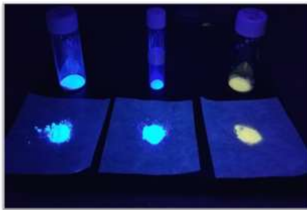
Fig. 1.1. Phosphor emitting light
